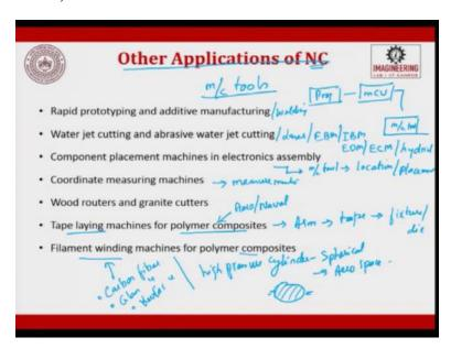
What are the other applications of NC machines? One is we were rapid prototyping and additive manufacturing. Again the machine tool is using the NC machines. Water jet cutting machine and abrasive water jet cutting machine uses NC. So, we are these are nothing but the machine tools, that is all. I have the program, I have a MCU, I have a machine tool.
