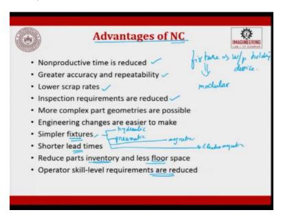
What are the advantages of an NC machine? The nonproductive time is reduced so that means to say, the loading, unloading time is reduced to a large extent, greater accuracy and repeatability can be achieved, lower scrap rates are generated, inspection required are since we have online monitoring itself say for example, we have a feedback device. So, which gives back to the MCU some instructions, this MCU start working and you get the required output.
