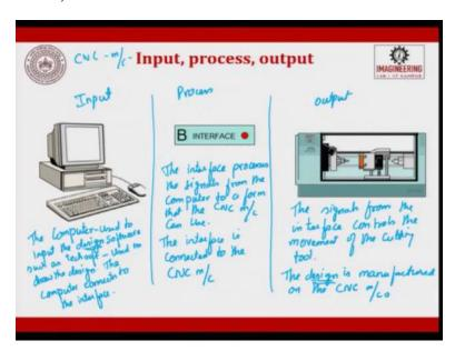
So, when we talk about CNC machines, CNC machines will have 3 inputs okay, 3 phases. So, one is input, you will have interface, you will have output. So, let us write down what is the function of this. The computer used to input the design software such as take whatever take I am just giving it as a tech soft, which is used to draw the design, the computer connects to the interface.
