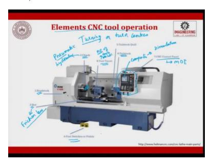
So, this when you look at the elements of a CNC machine this is what turning so this is nothing but a Turning machine there is a big difference between a turning machine, and a milling machine, turning machines are otherwise called as turn centres. So, in turn centres the work piece will rotate the tool will be approximately stationary, okay.
