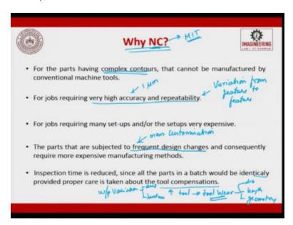
So why NC? For the part having complex contour that cannot be manufactured by conventional machine tool we always go for NC that is what I was trying to tell you after the World War, MIT was asked to make because the part complexity has increased. So, multiple parts have been integrated into single part so the geometry of the part of a single has become more complex.
