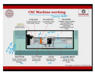
When you look at a CNC machine working, it will, you can see that there is a spindle, you will always have a light to aid you in the measurements or in see the execution, so there will be a light. So, there is a chuck, which holds the machine tool, so here it is pretty interesting you have fixed the tool here, the tool here and the work piece is attached to the tailstock, or I can put it, it is attached to the tool head in a normal machine. I am just trying to put another machine.
