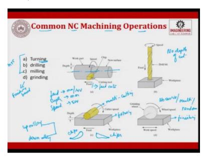
Some of the common NC machining operations are turning. So, with this is work piece, cylindrical work piece which is loaded onto a spindle. The spindle will be hydraulic and pneumatically done, and just like your conventional machine, you will have a feed which is given. So, feed leading to feed rates okay, with respect to time, then you will be given a depth of cut, all the other things are just like your normal machine, the terminologies are almost the same.
