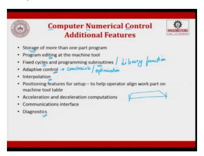
What are the additional features CNC machine has? It has a storage feature, it can allow you to edit feature, it has a fixed cycle and programming subroutines, fixed cycle programming subroutines if you are not able to visualize, you can think as a library function. So, library functions does a set of operations, where in which you give one or two parameters and get the entire operation done.
