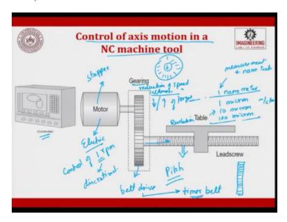
So, now let us see control of axis motion in a machine tool. So, controller we know, we know a motor, so this is ordinary electric motor, electric motor what happens you can control maximum of 1 rpm but really in a machine tool we are looking for accuracies. So, what are the accuracies of the table? We are looking at 1 micron accuracy, 10 micron accuracy okay, or 100 micron accuracy, today we are also started looking at 1 nano meter, nano meter accuracy.
