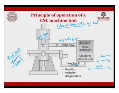
So, this is what I said last time, so it is a closed loop NC or a CNC machine tool, so you had a computer, you had a memory so the data was pulled out from the memory the program was executed, the data was given to the machine tool. The machine tool did execute whatever it was
