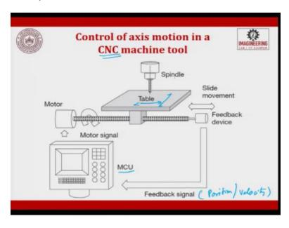
So, if you put that schematic diagram and if you fix it into a machine so you can see that table spindle and then you have a motor which is attached to a lead screw, lead screw in turn is attached to an encoder, which is a feedback device, okay this slide which is the spindle, table the slide movement is table movement, okay.
