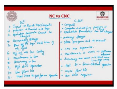
Now, let us see the difference between NC and CNC. So, this is numerical and this side we will write it as CNC. So, let us write down the difference 10 points, 1<sup>st</sup> point is input here is punched tape slash magnetic whatever it is. So, here it is computer, only computer. Next is, the program will always be punched on a tape. So, here it is used in a computer, so modification of program, modifying program is very easy, modifying is easy.
