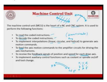
Next, we will see about machine control unit which was the second block in the sequence, in the schematic diagram of a CNC machine, which is machine control unit. Machine control unit is the heart of NC and a CNC system, machine control unit because the C whatever you had you are only punched words, letters, and symbols, but these words, letters, and symbols should be communicated to the machine tool, this happens by this machine control unit.
