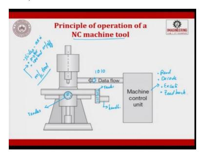
So, principles of operation of a NC machine tool, this is a machine tool, this is nothing but a machine we call it as a machine tool. So, you have MCU so this is where we saw read the code instruction and execute and analyze the feedback, all is done in this right, and then what you do is, what you give to the machine is nothing but the data, what is data? Data is nothing but 1 0-1 0 that's all, binary data you give it to the machine and then the machine moves accordingly.
