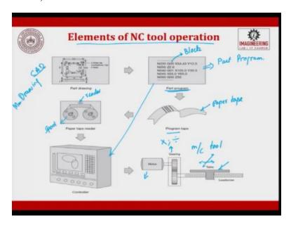
So, these are the elements of NC tool operation. Suppose, let us assume you have created this part drawing using CAD. So, this is, what in CAD? This is a drawing and this drawing is nothing but a manufacturing drawing, the difference between drawing and manufacturing drawing is drawing will have dimensions, manufacturing will have dimensions and tolerance, okay and it also will have references.
