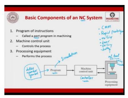
What are the basic components of a NC system? There are three basic components, one is program of instructions, so basically called a program, a part program in machining. So, this is the first basic component, a program for instructions. So, here is a program, so in programs you will always have letter, number and symbol, and this is used to controller which is used in machine control unit, okay.
