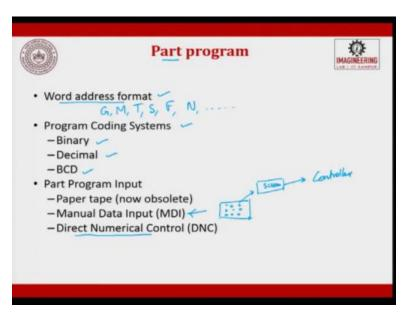
So, in a part program we will have word address format, we will have program coding system, it can be binary, it can be decimal, it can be binary converted to decimal, it can have part program inputs which is paper tape, MDI. MDI is you will have a console and in that console like a
