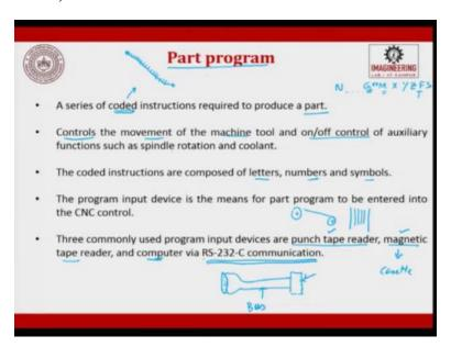
So, let us understand, what is part program? A series of coded instructions required to produce a part is called as part program. So, what are they? For example, coded informations can be the start of a line, it can try to have some codes, G codes, M codes, some X, Y, Z, F, S.
