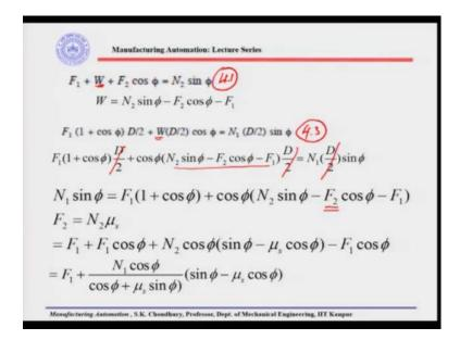
So, we have the equation 4.1 here; and from here, we will find out the W is equal to this, we have the equation 4.3 here. So, we take the value of W from the equation 4.1 and that value will be putting in the equation of 4.3.
