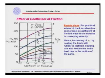
Next, what we said is the effect of coefficient of friction. We discussed that coefficient of friction is more, means, the conveying velocity of the bowl feeder will be more. So, there is a point in coating the track with rubber or some such material so that the coefficient of friction could be more. However, as we discussed last time that, it has to be decided based on the combination of the material of the track and the part that is being conveyed. So, this much we have seen last time.
