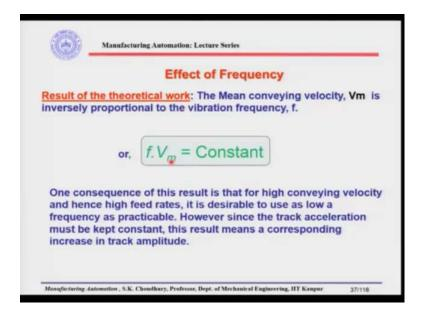
So, we have seen that, first effect is that  $fV_m$  remains constant; this is a theoretical work and because of that we said that if we have to increase the conveying velocity, the frequency to be selected should be as low as possible; that means, the amplitude of vibration has to be more, has to be as much as possible.
