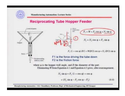
Now, our next feeder for the small parts, the one that we have discussed is the vibratory bowl feeder, the next feeder we will be discussing is the reciprocating tube hopper feeder. How the reciprocating tube hopper feeder works? Here is a feeder, there is a bowl and the mass of the parts, small parts are inside the bowl. Now, within the bowl, through the mass of the parts, there is a hollow tube which reciprocates, goes up and down.
