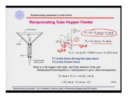
This will be the  $N_2\cos\phi$ . So, we have  $N_1$  which is resisted by  $N_2\cos\phi$  and it is also resisted by the  $F_2\sin\phi$ . This is the one which is  $F_2\sin\phi$ .  $N_1$  in this direction is resisted by  $F_2\sin\phi$  and  $N_2\cos\phi$  this is clear. So, this is the in the x-direction, this is in the y-direction. Now, let us see, if we say that point A here,
