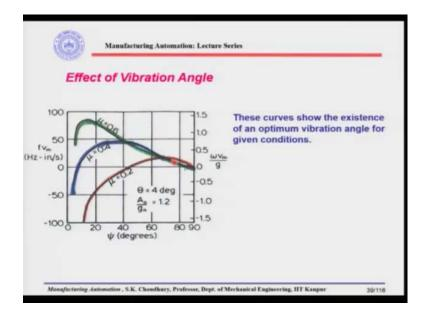
Effect of vibration angle: we said that there is an existence of the optimum vibration angle for different values of  $\mu_s$  that is the static coefficient of friction and as we are increasing the vibration angle, the  $fV_m$  increases, but it becomes stable after some time and then it decreases because of the same effect as we have seen in the case of track acceleration.
