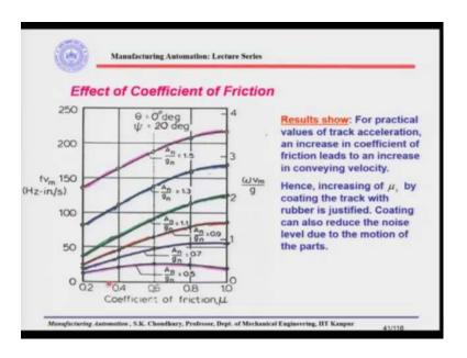
Here we have the coefficient of friction in the x-axis, we start from 0.2 and it goes up to 1, static coefficient of friction and in the y-axis, we have that  $fV_m$ , conveying velocity in Hertz inch per second and we have taken 0, 50, 100, 150 up to 250 of positive conveying velocity. So, these curves experimentally again have been taken for a  $0^0$  of track
