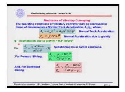
Then we said that the operating condition of the vibratory conveyor may be expressed in terms of the normal track acceleration and the normal track acceleration we said as  $a_0\omega^2\sin\Psi$ ;  $\omega$  is the angular frequency and  $a_0$  is the amplitude of vibration.
