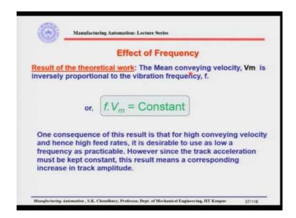
The result of the theoretical work says that the mean conveying velocity  $V_m$  is inversely proportional to the vibration frequency f. Now, what do you call it as a mean conveying velocity? It means, this is the speed of the part along the track of the vibratory bowl feeder and the track is inclined which is going spirally along the inside wall of the bowl feeder.
