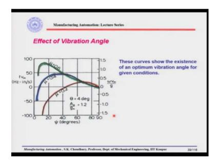
Next is the effect of vibration angle. Let us see what happens as the vibration angle is increased. Here x-axis is the vibration angle, y-axis is the conveying velocity  $fV_m$ . By the way, conveying velocity is given in Hertz inch per second. So, it is an American system because the data given by the American authors. So, it is inch system, in India of course, it will be centimeter or meter per second.
