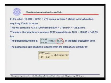
In that example we also said that the station breakdown basically happens because of the improper tolerances or improper parts which go into the assembly and it stops the machine, so the subsequent and the adjacent machines also get suffered.
