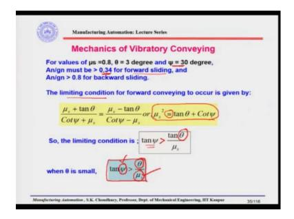
Now, for values of, for example,  $\mu_s$  is equal to 0.8, let us take a practical value suppose it is 0.8 and we have the track inclination angle as  $3^0$  and the vibration angle has  $30^0$ . In that case  $\frac{A_n}{g_n}$ , which is a normal track acceleration, must be more than 0.34 for forward sliding, we are getting it from here as you understand.
