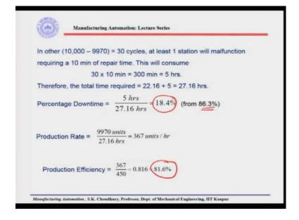
So, through this example I wanted to show that the machine breakdown has to be considered while discussing or while taking care of the production flow line for the assembly.
