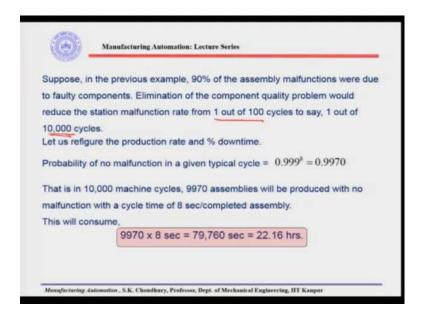
So, if we can improve the product quality, in that case, as we have taken in that example, that suppose we have instead of 1 out of 100 we have 1 out of 1,000 cycle malfunctioning. Then it is improving drastically again and the percentage downtime reduces to 18.4 from 86.3%. I am just reminding you, the production efficiency goes up to 81.6%.
