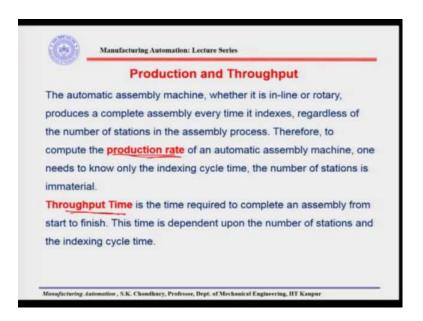
We have seen that the throughput is the time taken for an assembly to be completed. And also one fact that I would like to once again repeat that in an assembly line whether it is in-line or the rotary one, each time it indexes we will get one complete assembly, this you have to keep in mind.
