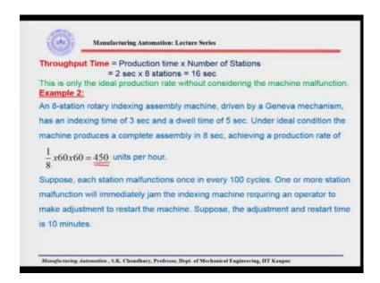
Therefore, the throughput time will be equal to the production time into the number of stations. So, number of stations will be immaterial while considering the production rate. Whereas, in considering the throughput time we have to have the production rate into the number of machines/ number of stations.
