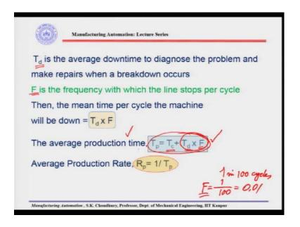
Let us say the line stops per cycle once in every 100 cycles. So, if 1 in 100 cycles, then,  $\frac{1}{100}$  is the frequency. So, this is 0.01. So, let us say this is the F which is the frequency with which the line stops per cycle let us say once in 100 cycles or it may be once in 10 cycles, once in 1000 cycles that depends and on which factors we will discuss later.
