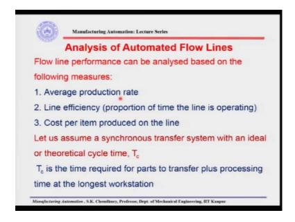
Now, the automated flow lines can be analysed based on the average production rate, as we said, based on the line efficiency and the cost per item produced on the line. These are the topics that we discussed last time. I said that the line efficiency is important because this will dictate us or this will show us what is the proportion of time the line is operating. The rest of the time the line is down, and why the line becomes down that we will discuss now.
