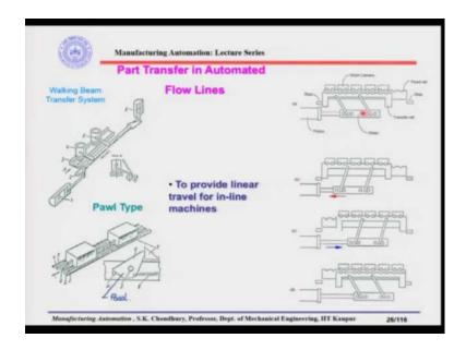
Welcome back. Now, let me remind you that we were discussing the part transfer in automated flow lines. You can see from the diagram here. This is for the linear travel from one work place to another work place for any part or for any sub assembly if it is an assembly flow line. So, this system is called the walking beam system; that means, as if it is walking.
