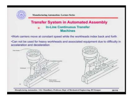
Next is a transfer system in automated assembly. Here it is the in-line continuous transfer mechanism, as I was telling you that in-line continuous transfer mechanisms there you cannot use the bigger head or the bigger work heads because they will have the inertia. Look at this example, here we have the feeder, where we have the small parts which are being fed to the machine which is being processed or assembled.
