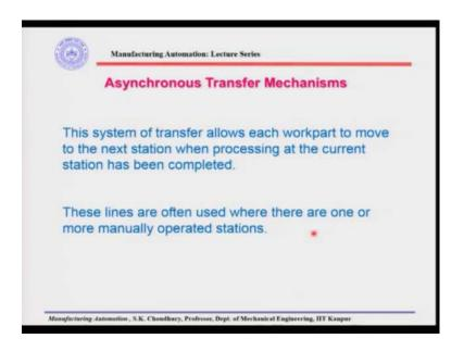
Now, the asynchronous transfer mechanism. As I discussed earlier, this has eliminated the disadvantage of the earlier mechanisms where the adjacent machines are affected if the machine breakage happens or if the processing time of the adjacent machines is different.
