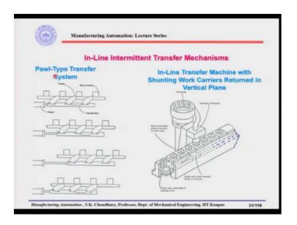
Here is another example of the pawl type transfer mechanism. This is similar to the one which we have discussed earlier and like the walking beam system. So, these are the pawls, these are the pawls which are spring loaded and while this works with the work carriers, when it is coming back, they will actually go under the parts and they will be dipped so that it could come back to the initial position.
