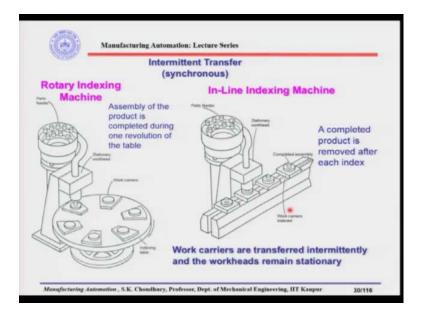
Here is another example. This is a rotary indexing machine and normally the rotary indexing machines are driven, as I said, by Geneva mechanism, so that the parts can be moved from one position to another position. And dwell for some time. Dwell for some time means it will stop for sometimes so that, this work head can actually make the process either it is a processing station or it can be an assembly station.
