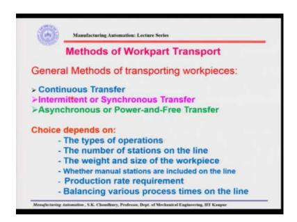
Let us see the methods of work part transport. The general methods of transporting work pieces are the continuous transfer, intermittent or synchronous transfer and the asynchronous or power and free transfer. Let me explain what are those things. Continuous transfer is where the parts are being transmitted continuously, they are not stopping.
