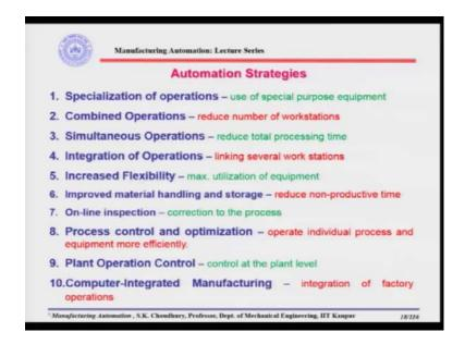
So, first point is the specialization of operation, that is the use of special purpose equipment which will be able to perform one job precisely, and that machine will be specially used for that particular operation. Therefore, we are calling that machine as a specialized machine, for specialization of operation.
