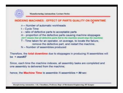
Let us discuss first the indexing machines and the effect of part quality on the downtime. Meaning that if we have different quality of parts then how the downtime of the machine will behave; that means, we will find out the down time. Now in this analysis let us say n is the number of automatic work heads, t is the cycle time, x is the ratio of defective parts to acceptable parts. What does it mean?
