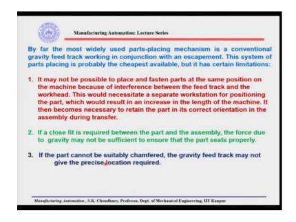
By far the most widely used parts-placing mechanism is a conventional gravity feed track working in conjunction with an escapement. This system of part placing is probably the cheapest available. Example I have shown to you earlier. So, those are the conventional gravity feed tracks in conjunction with an escapement.
