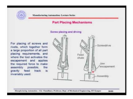
Let us see what are the part placing mechanisms. Normally, they are the manipulators, they are the robot hands and so on. However, look here this is the diagram which is showing the screw placing and driving. Here in this diagram what is shown is that from the feed track the parts are coming in here. So, this is the jaw or this is the screw drive for example, this can go up and down.
