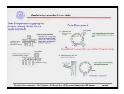
The next escapements we can see from here, this is an example which is the slide escapement supplying two or more delivery chute from a single feed chute. Look at this example here; what we are saying is that there are three parts from the feeders. These three parts are coming in this example and delivered to three feed chutes. In this example what we are doing is one we are taking from one feed track and it is being delivered to once to this feed chute and another to this delivery chute.
