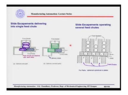
Well, let us see the other examples. In this case, slide escapements delivering into single feed chute. Here these are the parts coming from the feeder either it can be horizontal feeder or it can be a vertical feed delivery. And, the part when it is coming at the end of the feeder, there is a cross slide here and this slide can reciprocate. While the slide is going to this side, it will take one part from the feed track and deliver to the machine. So, this is going to the assembly machine.
