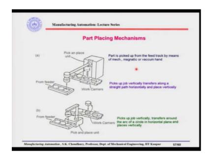
Another part placing mechanism or other part placing mechanisms as I said that these kind of robotic arm or manipulator can be used. So, in this part is picked up from the feed track by means of mechanical, magnetic or vacuum hand. So, this is the manipulator or the robot arm and it has an end effector. It can be a mechanical gripping or it can be a magnetic if the parts are of ferromagnetic material or it can be a vacuum hand.
