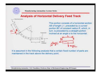
Now, let us have an analysis of the horizontal delivery feed tracks and let us see how the horizontal delivery feed tracks are designed. Let us take an example that this is the feed track that we have and here we have the inclined portion; inclined straight portion we have the curved portion and then there is a straight portion.
