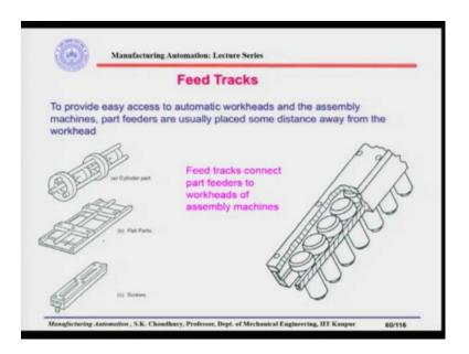
Now, we have shown some of the part feeders for a feed tracks. So, these kind of feed tracks for example, you have seen that this is for cylindrical part, for flat parts, for parts headed parts which are hanging in the slot.
