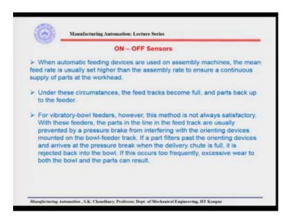
Let us discuss one thing which is interesting which is called the ON-OFF Sensors in the feed track. See what happens is when automatic feeding devices are used on the automatic assembly machines. The mean feed rate is usually set at a higher rate than the assembly rate to ensure a continuous supply of parts at the work head. So, I told you this thing earlier also, that work heads should not starve because that will then effect the other adjacent work heads.
