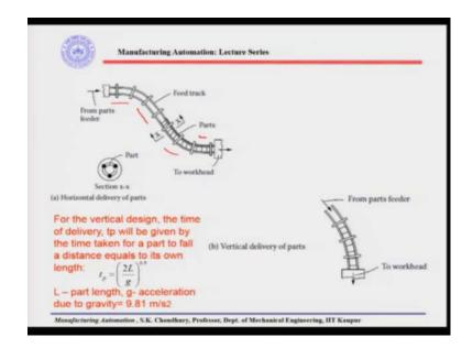
On then we said that the part feeders sorry feed tracks are normally of two types; they can be of the vertical delivery of the parts, where the parts are fed with the gravity and in that case that the time taken for a part to fall will be equal to 2 L by g root over because this is the acceleration due to gravity that we are using to deliver the parts.
