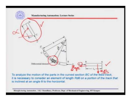
Let me going ahead show you this that here in this AB, we have this F 1 if it is a free body diagram, free body diagram of the entire feed track; so AB which is the straight part of length L 1, this has then F 1 here and F 1 reaction here. So, therefore, if we have
