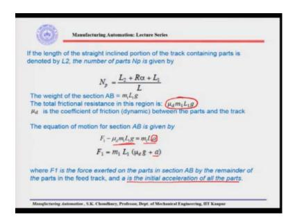
Now, if the length of the straight inclined portion of the track containing parts is denoted by L 2 this is the L 2 and the length of the straight path is L 1, and the curved portion has a radius of R and this angle is alpha that is starting of the curve portion and the end of the curve portion.
