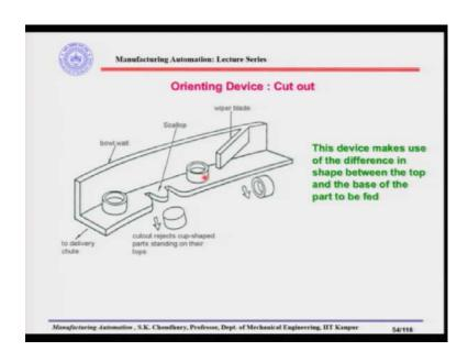
We have seen the parts with the heavier side and the open side. We saw that the scallop is very suitable for such parts to go through when it is coming with the closed side or the heavier side down.
