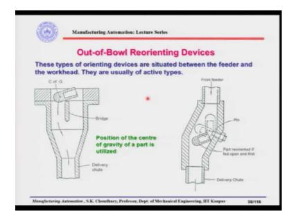
Now, let us discuss the out-of-bowl reorienting devices and I will remind you that out-ofbowl reorienting devices are always used outside the vibratory bowl feeder. And they are normally active orienting devices because had it been passive orienting devices, the parts will be rejected, but the parts cannot go to the bowl back because these parts have already come out of the bowl.
