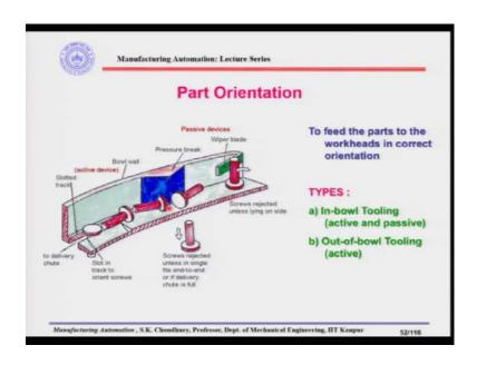
For example, we have discussed parts like as you can see here, the headed parts. So, for the headed parts it is better when the parts can actually be fed hanging on the head, if that orientation is the desired orientation.
