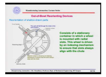
Here is an interesting out of bowl reorienting device and these devices are used for cup shaped parts like this; here is a kind of a cup shape.
