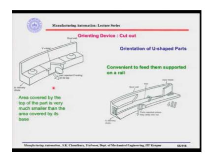
Next let us say the orienting device here which is a cut out which is quite similar to the scallop. But here what we use this for is, for a part where the diameter at the top and the diameter at the bottom are quite different. So, the are conical in shape like this as it is shown here; so, through the track, when the parts are coming, these parts will be coming either with the bigger diameter down or with the bigger diameter up.
