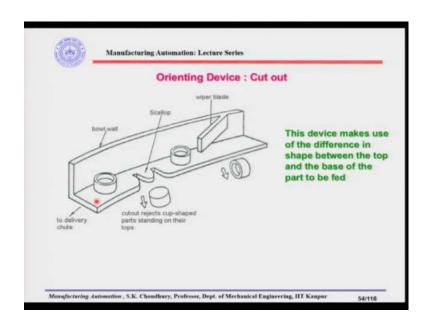
The next one is an orienting device which is a new orienting device, as shown here. This is the scallop. Let us say this is a track, and this is the bowl feeder wall and this is the sector of a vibratory bowl feeder. Now, through this we have to take the parts, we have to feed this kind of parts. And this device makes use of the difference in shape between the top and the base of the part to be fed. So, the part is like this.
