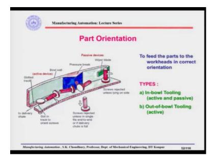
Now, our next topic, we will be discussing the part orientation. And earlier as I discussed, the parts have to be fed to the automatic assembly machines from the bowl feeders in a right orientation. So, there have to be some kind of orienting devices, so that the parts could be fed to the right orientation in case the parts are not coming in the right orientation at the bowl feeder exit.
