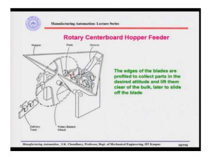
So, let me remind you that last time we have discussed the rotary centerboard hopper feeder. And, in here the design, as we said, that there is a hopper and the edges of the blades which are rotating within the mass of the parts located at the base of the hopper, are profiled to collect parts in the desired attitude and lift them clear off the bulk, later to slide off the blade.
