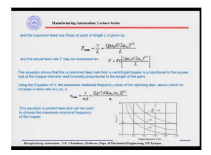
And this divided by the part length will give you the maximum feed rate. Therefore, we said that the maximum feed rate is proportional to the velocity and inversely proportional to the part length.
