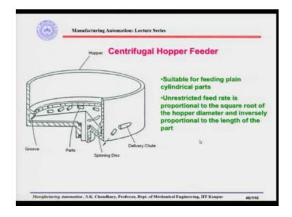
Next we discussed the centrifugal hopper feeder, where we have the base which is rotating and during the rotation the parts are being imparted a centrifugal force. Because of the centrifugal force, the parts are nested in the slots which are located at the outer periphery of the inner disk and when these slots will be aligned to the delivery chute, the parts will be coming out one by one.
