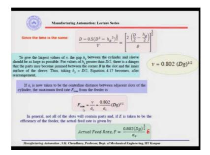
So, the critical velocity can be found out from the distance travelled; that means, the distance while moving from this position to this position, the part is moving horizontally to a certain distance and at the same time the part is falling vertically; that means, moving down.
