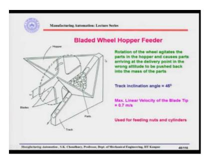
The next hopper feeder is the bladed wheel hopper feeder, this is another design; there are various designs of the hopper feeders. You have to select one of them depending on the type of your production, depending on the type of the part that you are actually feeding.
