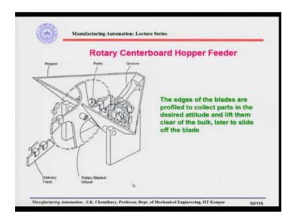
Here is another centerboard hopper feeder. Tthis is called the rotary centerboard hopper feeder and here the principle is different than the one that we have discussed. See they are very similar to the look as the bladed wheel hopper feeder where the blade is not selecting the parts, its agitating the parts; whereas, in this case, what happens, the same kind of a bowl hopper and at the base of the hopper we have the parts.
