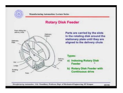
After that we have discussed the Rotary Disk Feeder. In here we have the bowl and the base of the bowl rotating and at the base of the bowl we have the slots and those slots are protected by the ledges here and by a stationary disk, so that when the parts will be nested in the slots, the parts will not be falling down in this direction or in this direction.
