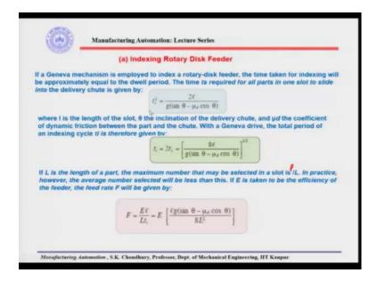
Here, we can find out the maximum feed rate or the mean feed rate by finding out how much time it is taken, if a Geneva mechanism is involved, we consider that the index time and the dwell time is the same. So, this can be found out from the  $\frac{2l}{g(\sin\theta - \mu_d\cos\theta)}$ , which is  $t_s^2$  if you remember, we have done that earlier.
