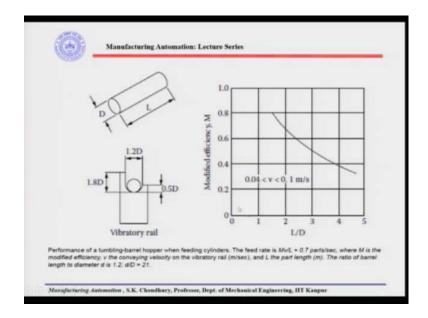
Here is one example of the kind of a part that is fed through the vibratory rail, length and the diameter given. So, vibratory rail when you are actually selecting, if the diameter of the part is this. So, this is 1.2 dia and this is 0.5 diameter. This is the shape of the vibratory rail, that you can design depending on the part that you have with a certain diameter and with a certain length.
