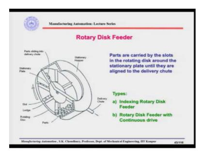
Well, the next feeder is the rotary disk feeder. This configuration is given in the pictorial view here. Parts are carried by the slots in the rotating disk around the stationary plate until they are aligned to the delivery chute. Now, here there is a stationary hopper and the base of the stationary hopper rotates. In the base of the stationary hopper there are slots and those slots are protected by, as you can see, this is protected by the ledges, here are the ledges.
