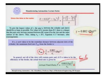
Now, since the time is the same, meaning that at the same time the part is moving horizontally as well as vertically. Therefore, the time taken for the part to move horizontally we can equalize with the time taken for the part to move vertically and we can find out from this equation the velocity at which the part will fall through the gate will be equal to  $0.802\sqrt{Dg}$ . D is the gate diameter or the path diameter, g is the gravity.
