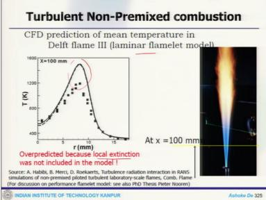
So, now this is another for the same using this flamelet model, how we get the radial distribution of the temperature of these things. So, there are some over predictions of the local extension because these temperature profile is over predicted as the flamelet model does not take into account the local extinction. Okay. So, this is what give you an idea if you look at this literature, this will give you an idea of the different issues of flamelet model and all these things.
