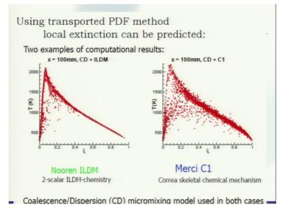
This is an example which will be picked up from a transported PDF calculation for the local extension that was predicted, so this is using natural gas.
