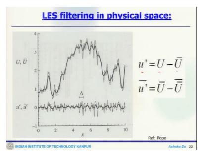
This is typically how a signal is represented because if you have a fluctuating component, which can be obtained from the instantaneous component minus the union value.
