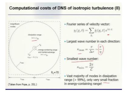
Now, we can estimate the competition cost for an isotopic turbulence like you have this situation where dissipation range would be at this. So, then free a series of the velocity vector can be expressed like that. So, we can find out the large wave number in each direction that is phi by delta x which is order of phi by eta. Now, smallest to wave number that would be 2 phi by L and he said majority of the most dissipation range.
