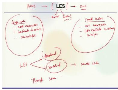
Now, one hand you had so this is an intermediate solution between RANS and DNS, because these DNS you resolved for all the scale, RANS you model for all the scale, in LES what do you do you model for large scale structure a resolve for large scale structure and only model the small scale structure. So, essentially, theoretically LES can go towards DNS, if you are modeling part. So, there are 2 parts, 1 is the resolve part another is the model part.
