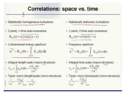
So, this if you combine things here so, one case you have a statistically homogeneous turbulence, you can have statistically stationary turbulence your 2.1 time covariance is calculated like this, 1.2 time covariance is calculated like that, because this is statistically stationary turbulence. Then one dimensional energy spectra will get you back the u prime square this frequency spectrum which will get you.
