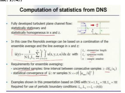
So, this is fully developed channel flow. So, this will have be statistically stationary and also statistically homogeneous in both X and Z direction. So, the Reynolds average can be based on a combination of ensemble average and linear line average like this, where  $L_z$  is span wise length,  $L_s$  is stream wise length, alpha is sample number. So, the requirement for the ensemble averaging if they are uncorrelated sample, then the time interval between the consecutive scale.
