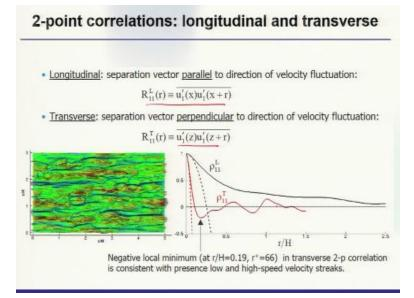
Now, similarly, you can have the longitudinal and the transverse variation. So, the longitudinal separation vector parallel to the direction of the velocity fluctuations where  $R_{11}$  is defined like this and then go to transverse this will be transfer which is perpendicular to the flow and there variation are different the longitudinal variations is like this where the transverse one initially quite steep and then it decays.
