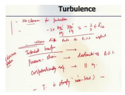
Some comments one of the important is that for production term there is no closer required then microstructure they are except close to the wall they are isotopic, so, that will approximate like this then also microstructure level negligible contribution to the reynolds stress. So, viscous, dissipation rate of reynolds stress neglected. Now, these are some of these things, but there are certain other problems, problems like turbulent transport.
