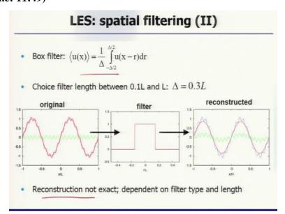
So, there is a different kind of filters which are available, one can see there is a box filter then originally the signal looks like this then if you put the filter then it comes like that. Construction obviously not exact, but it depends on filter type and the length which has been used.
