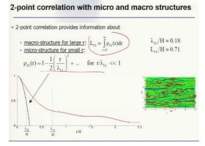
Now, when you look at the 2-point correlation so, this provides the information about macro structure for large L which is the integral length scale and then microstructure are small r which is like this. So, if you plot these things, this is what it buries, this is again for that channel flow that we had this is I mean one can do this for.
