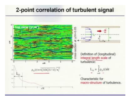
For the said 2.1 time auto covariance for statistically homogeneous terminals, again if you look at the same calculation of the channel flow, you can see if you plot this normalized variable, this is how it actually vary and from here one can define the integral length scale, the integral length scale would be the integration of rdr. So, this is a characteristic for macro structure of turbulence where you get an estimate of your integral landscape.
