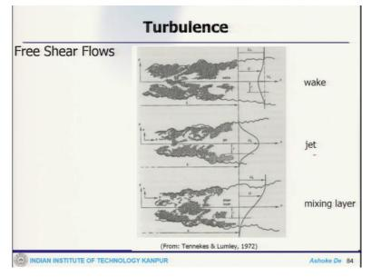
Now, this is an example of free shear flow where you see a mixing layer where two different layers they are mixing. Different kind of eddies that form and the velocity profile is shown. These are some example of free shear flows.
