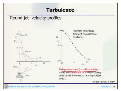
When we look at the round jet, as we go along with the axial distance, the velocity profile is shown for this. This actually gives an idea that this is self-similarity: mean flow in variant of x when scaling with centreline velocity. This is an important hypothesis.
