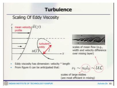
Now, the scaling of eddy viscosity. If l is the size of the turbulent eddy, which is having a velocity scale of u(l) and the picture of the shear layer is shown above. The Eddy viscosity is order of  $v_t \sim u_0 l_0$  and for the large scale it is  $v_t \sim U L$ , that is for macro structured scale for the large eddies, which allows more efficient mixing.
