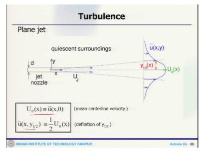
Now, we see a planar jet, there is a jet nozzle and from where the jet is injected and further downstream, we can see how the profile looks like.
