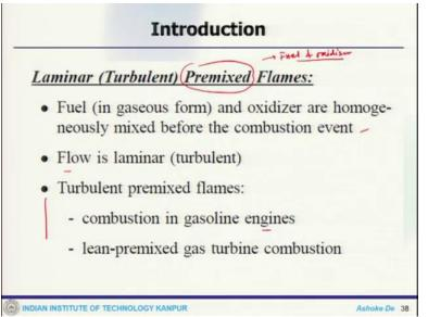
Now if we get to the details of this laminar or turbulent pre-mixed flame what it exactly it is so as the name suggests the pre-mixed that means, your reactants are of two types one it will have the fuel so that means your fuel and oxidizer. So, they are pre-mixed before they are injected into the combustion chamber. So that is why the premixed comes into the picture where things are previously before injection they are mixed.
