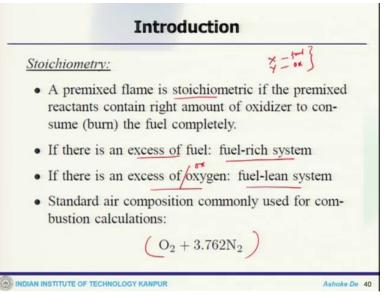
Now another definition is that when you talk about the pre-mixed flame is the stoichiometry. So, typically the pre-mixed flame is stoichiometric if the flame reaction contents right amount of oxidizer to consume the fuel completely that means if I mix X amount of fuel with Y amount of oxidizer? So the proportion is rightly mentioned so that you get stoichiometric situation. If for example, the fuel is excess then one can say it is fuel rich system.
