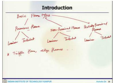
Now we can come to some of the basic flame types. So the basic flame types; so one of the system could be pre-mixed flame that is one of them then one can have non-premixed flame. So we will talk about these flames in details that so now we are getting into the classification of different flame types. This could be one of these partially premixed flames. So, these are the three primarily broad categories of flame where you have one premixed non-premixed, partially premixed.
