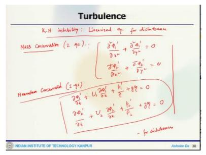
Now we can formulate the linearized equation for disturbance so still we are doing KH instability this is linearized equation for disturbance. So from mass conservation equation we get 2 equations one is:
