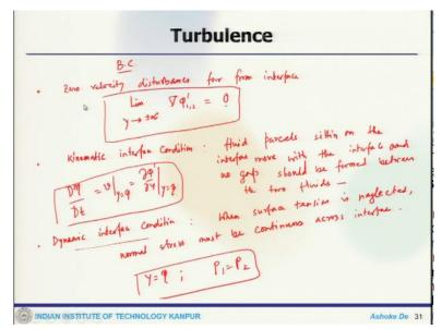
Now we need boundary conditions which are quite important. Number one we can have 0 velocity disturbances far from interface that means one can write:
