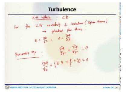
So here we are talking about K H instability. So we derived the governing equation now for flow with no viscosity and irrotational which is a Kelvin theory this is a flow it is insulation potential flow theory which gives you:
