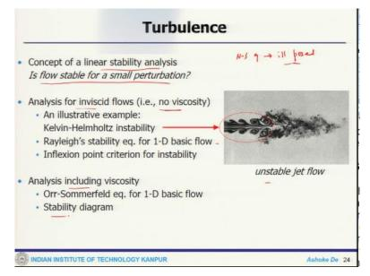
Now we have already said that for a turbulent flow the Navier stokes equations are ill-posed that because if we make some small perturbation to the initial condition or boundary condition the flow does not remain any more stable. So this is the where we can use our concept or linear stability to see whether the flow is stable or not for some small perturbation. Now this is quite important to identify the zone where you can see the stable flow field and the zone where it is unstable.
