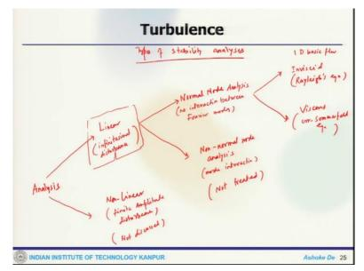
So the types of stability analysis one can do if you start write bottom here the analysis let us say this can go to one direction where it is a nonlinear. So which is something called finite amplitude disturbance or other one is the segment where we can say it is a linear that means infinitesimal disturbance okay. Now we will do or restrict our analysis for the linear system only, so this one will not going to be discussed.
