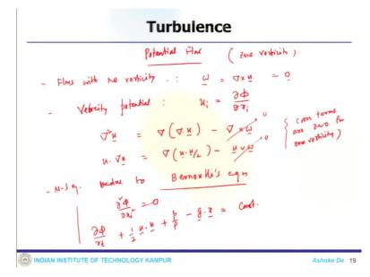
Now, we will go back a little bit and start with some simple system like potential flow, so which means that is 0 vorticity so, the potential flow means flows with no vorticity so, that means there is no stretching of fluid parcel neither the rotation of the fluid parcel so, which means  $\omega$  is 0 so, you can have a velocity potential and one can define  $u_i$  as:
