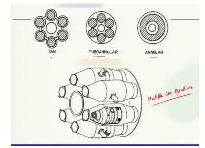
So, now we also talked about some combustors. Basically, specially which is used in your GT applications and these combustors are of like one could be can type, one could be annular type, turbo annular type and this is another schematic of your multiple can here you see 1 2 3 4 5 these are multiple can operation. So they do take part in the power generation of the thrust generation process.
