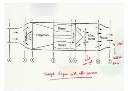
Now, this is another schematic or cut section of the engine with afterburner. So, this is a turbo jet engine with afterburner. So there you see the difference here, you have typically here comes through diffuser, then compressor, then goes through the combustion chamber or the burner then you pass through the turbine where the expansion takes place. And then after that you have afterburner which is second level of combustor which is there, where you add more fuel there.
