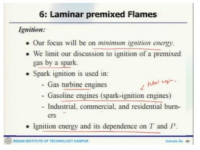
Now we will move to the third point which is ignition. So, what here we wanted to look at is that are the objective is that to on minimum ignition energy that means, what is the minimum energy that is required to move the reaction forward. So, that is what is quite important. Now we limit our discussion to the ignition of a premixed gas by spark only. And if you go to the textbook, you will find there are other methods also or other ways to do that analysis.
