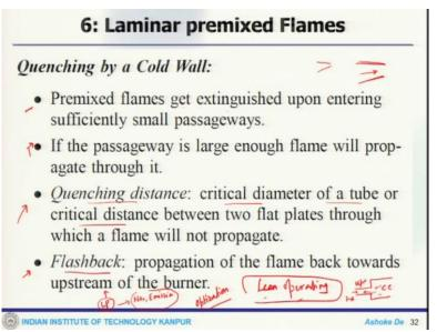
Now, we will go one by one and look at what happens when quenching takes place by a Cold Wall. Now, the flame front the especially the premixed flame front can get extinguished when it entering sufficiently small passage that means, if you allow to pass through various small passage, then it can quench that is one of the ways it may possibly happen if obviously the flip side of it is that if the passage is large enough or broad enough, then the flame will propagate through it. Okay?
