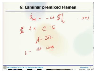
Now, through the slab of the wall, the heat loss by conduction, which follows the furious law. So, we can get the combustion heat loss which is nothing but:
