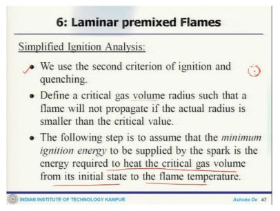
Now, how we go about the simplified ignition analysis, we use the second criteria of the ignition and quenching so, that is our first thing when we define a critical gas volume radius such that the flame will not propagate if the actual radius is smaller than the So, that means, we will define something like that there is a critical radius beyond that there will be flame temperature.
