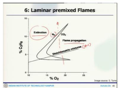
Now, similarly, one can look at this is propane and there is a representative curve for propane when it is with the percentage of oxygen. The reaction goes on what happened to that mixture. So you can see this side of the curve region, this is your nitrogen formation curve which goes like this to the percentage of oxygen and this is your stoichiometric mixtures  $\varphi$  1 condition this is your CO<sub>2</sub> formation.
