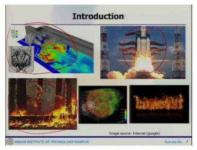
Now, there are some more example and that one can see. This is another example of your gas turbine combustor. This is a very, very specific unit. I mean, that is and just an example because different gas turbine engine has different kind of combustion. So their geometry would be different. But this one shows you there is a swirling been there. Then the fuel is liquid fuel is injected so this sort of a kind of flame instantaneously that you can see.
