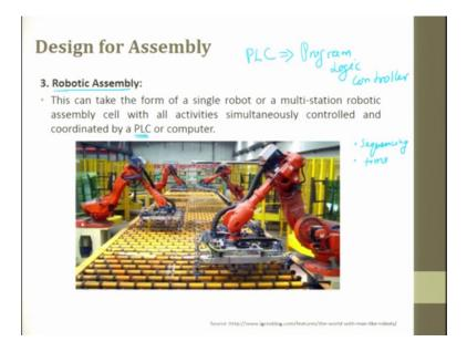
This is robotic assembly; so this can take the form of a single robo or a multiple station robotic assembly cell with all activities simultaneously control and coordinated by a PLC; PLC is Program Logic Controller. So, which tries to say first this operation to happen that operation to happen third operation forth operation fifth operation and if at all there is any problem in the first or second it goes to an emergency stop.
