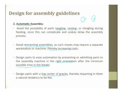
When we talk about automatic assembly line the first guidelines is avoid the possibility of parts tangling nesting and shingling during the feed. For example, when we try to feed it is said as automatic assembly. So, when we try to do automatic assembly you are replacing the man. So, when you replace the man the parts which is there in the tray which I was talking to you now has to come through a shoot or a conveyor.
