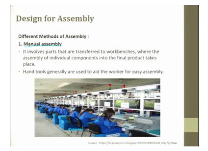
So, different methods of assembly these are called as manual assembly. So, in manual assembly what happens; you can have a conveyor belt. This conveyor belt can be moving from station to station to station and people are involved in doing assembly so. In fact, when the placing of parts and then they the hydraulic ramp to push the part inside or they just do assembly and do soldering along the assembly line.
