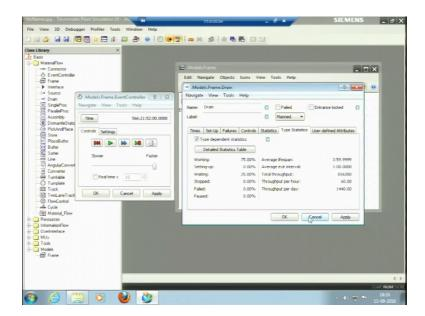
If I right click here and open I can see my throughput here in a type statistics in the type statistics. So, it has produced 1440 pieces throughput per hour is also given, throughput complete for 566 days it has run for 566 days ok. So, it has produced 816350 these many number of pieces ok. So, I can see the throughput.
