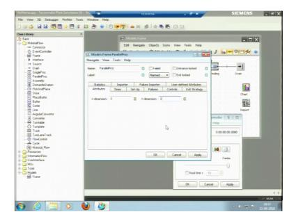
You know if I put parallel process and right click here and open parallel processes when we have exactly same machines for instance we have four drilling machines of same make which is having saying processing time and same setup time and what we need not to put the four machines in parallel specifically four single processes in parallel. We can pick one parallel process because other parameters are same the attributes of this specific process is same.
