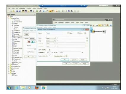
So, if failure happens if actually the processes failed that is the kinetic abilities stop it takes about 1 minute to repair that. So, these attributes we can select. So, I will keep it
