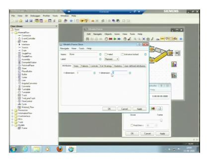
Store is a kind of a longtime storage. So, you can see this is the capacity 3 into 3 9 pieces can be stored here ok. I can just change the capacity do the number which I like not which I like which is actually required in the process. So, this is to I am deleting this one.
