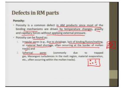
Next defect is porosity; porosity is a common defect in additive manufacturing products since more of most of the binding mechanism are driven by temperature changes, gravity and capillary forces without applying external pressure. Porosity can be found as irregular pores and spherical pores, irregular pores due to shrinkage lack of binding fusion or melting or material feed shortage.
