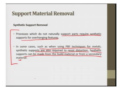
Next is synthetic support material removal, the processes which do not naturally support pass required synthetic support for overhanging features. In some cases such as when using powdered bed fusion techniques for metals synthetic supports are also required to resist distortion. Synthetic support can be made from build material or from a secondary material.
