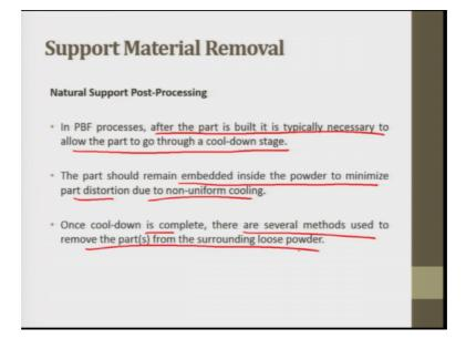
Now, in powder bed fusion process after the part is built it is typically necessary to allow the part to go through the cool down stage. The part should remain embedded inside the powder to minimize part distortion due to the non-uniform cooling the cool down time is dependent upon the built material and the size of the other parts. Once cool down is complete there are several methods used to remove the parts from surrounding loose powder.
