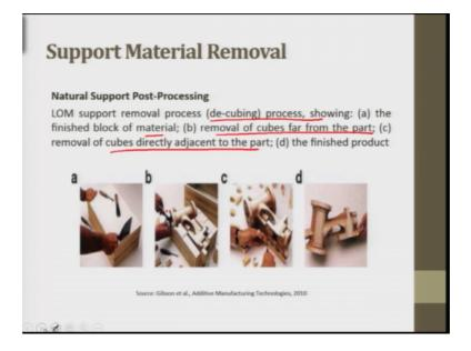
You can see the laminated object manufacturing support removal process that is de cubing process showing the finished block of material, then second part is b part is removal of the cubes far from the part this is the cube far from the part b a being removed. And these are the cube which are close to the part just adjacent to the part that is part c, then the finished product is taken. So, this is natural support post processing.
