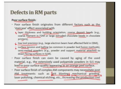
Next as a defect also we can say poor surface finish; poor surface finish originates from the different factors such as staircase effect as I explained which is associated with layer thickness and building orientation course deposit beads. For example, course filament in FDM or large extruded chocolate beads in chocolate printers.
