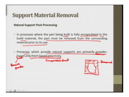
Now, natural support post processing in processes where the part is being built this fully encapsulated in the build material the part must be removed from the surrounding material prior to its use. The processes which provide natural supports are primarily powder based and sheet based processes.
