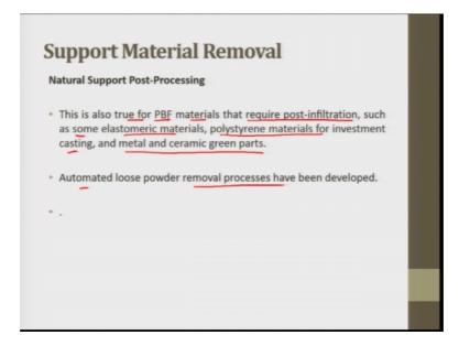
So this is also true for powder bed fusion material that required post infiltration such as some elastomeric materials polystyrene materials for investment casting and metal and ceramic green parts.
