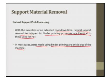
Now, with exception of an extended cool down time natural support removal technique for binder printing processer are identical to those used in powder bed fusion. In most cases parts made using binder printing are brittle out of the machine. Thus until the parts has been strengthened by infiltration. The parts must be handled with care because they are brittle.
