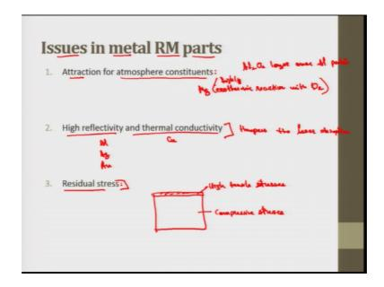
There are certain issues or challenges those come in specifically in metal rapid manufacturing parts. Number 1 is attraction for the atmospheric constituents, number 2 is high reflectivity and thermal conductivity, number 3 is residual stresses.
