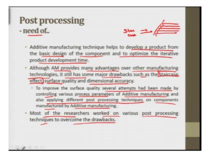
Now, post processing need of additive; manufacturing techniques helps to develop a
