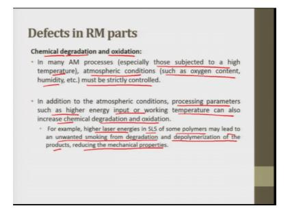
Next defect is chemical degradation and oxidation. In many additive manufacturing processes especially those subjected to a high temperature atmospheric conditions such as oxygen content, humidity etcetera must be strictly controlled. So, this is required to prevent or minimize degradation and oxidation.
