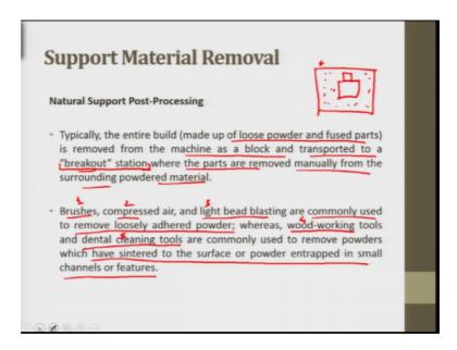
These methods can be all different they can be vibratory methods or the manual powder removal. So, typically entire built made up of loose powder fused parts is removed from the machine as the block and transport it to a break out station with the parts are removed manually from the surrounding powdered material. So, what happens this is this complete box, let me say this bottle is manufactured here this complete part is taken to the breakout station where they will remove this powder ok.
