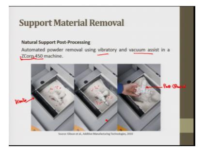
So, this powder this powder that is shown in this figure is a natural support. So, this is are mostly the powder based and sheet based as I said the material that is surrounding the build or the part that is being manufactured. So, this natural support in powder bed fusion
