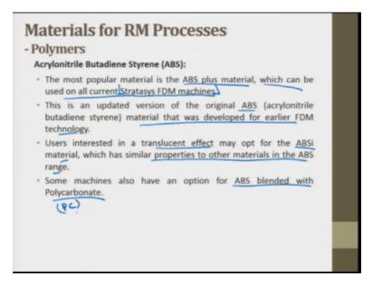
The most popular material is ABS plus material, which can be used on current stratasys FDM machine. This is a company that has these machines it is an updated version of the original ABS material that was developed earlier FDM technology. Users interested in a translucent effect may opt for ABS material, which has similar properties to other materials in the ABS range. Some machines also have an option for ABS blended with polycarbonate which is PC also known as PC.
