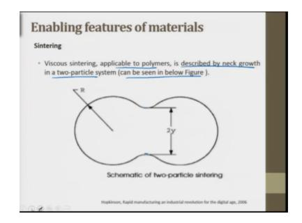
So, time and sintering parameters are to be defined. There are certain parameters or certain ways the sintering happens. One of the ways is now this is viscous sintering. That is applicable to polymers, this is it is described by neck growth in a two particle system and can be show in a below figure, this is viscous sintering in which this neck is formed this is radius of the particle two particles are sintering. So, this is the neck that is formed.
