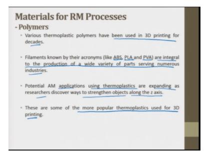
Next is polymers various thermoplastic polymers have been used in 3D printing for decades filaments known by their acronyms ABC PLA, PVA are integral to the production of a wide variety of parts serving numerous industries. Potential additive manufacturing applications using thermoplastics are expanding as researchers discover ways to strengthen objects along the z axis.
