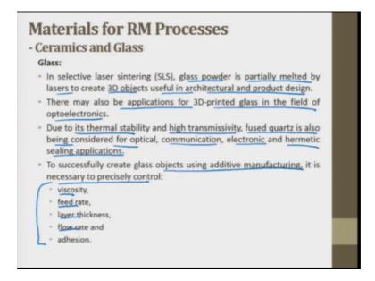
Next is glass; glass is another material in selective laser sintering, glass powder is partially melted by lasers to create 3D object useful in architectural and product design. There may also be applications for 3D printed glass in the field of optoelectronics. Due to it's thermal stability and height transmissivity fused quartz is also being considered for optical, communication, electronic and hermetic sealing applications.
