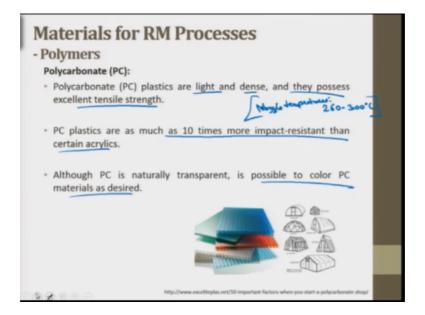
Polycarbonate plastics are light and dense and they possess excellent tensile strength. Polycarbonate plastic are as much as 10 times more impact resistant than certain acrylics. All though PC is naturally transparent it is possible to color polycarbonate materials as desired, carbon reinforced polycarbonate plastic are strong and heat resistant enough to use in manufacturing intake, manifolds and other parts subject to high temperatures.
