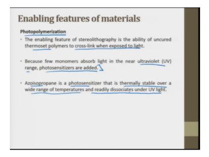
Next enabling feature for materials is photo polymerization; photopolymerization. This is discussed in detail in the previous lectures when we discussed photo polymerization based rapid manufacturing process is. The enabling feature of the stereolithography is the ability of uncured thermoset polymers to cross link when exposed to light this is just the recall.
