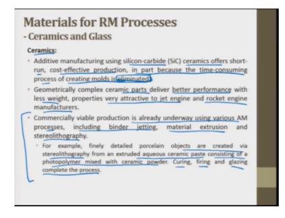
Next we have here is ceramics and glass; ceramics and glass or another additive manufacturing materials, so additive manufacturing using silicon carbide ceramics offers short run cost effective production in part because the time consuming process of creating molds is eliminated. So, the molds are not to be made, so these are cost effective. Geometrically complex ceramic parts deliver better performance with less weight, properties very attractive to jet engine and rocket engine manufacturers.
