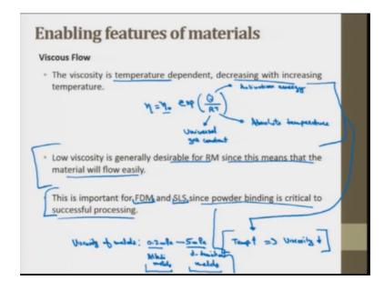
In viscous flow, viscosity is temperature dependent, decreasing with increasing temperature. Both polymers and liquid metals for there is a general relation this eta can
