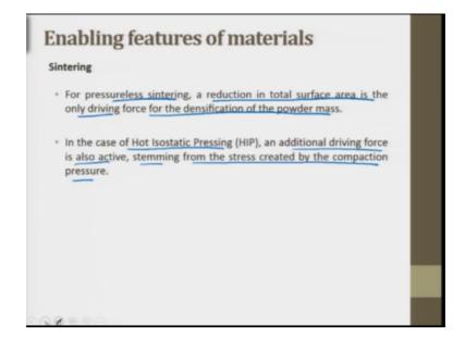
So, rather than solid state sintering that is being described here pressureless sintering is also one of the ways. For pressureless sintering a reduction in total surface area is the only driving force for the densification of the powder mass. In the case of HIP Hot Isostatic Pressing and additional driving force is also active, stemming from the stress created by the compaction pressure. So, this is sintering.
