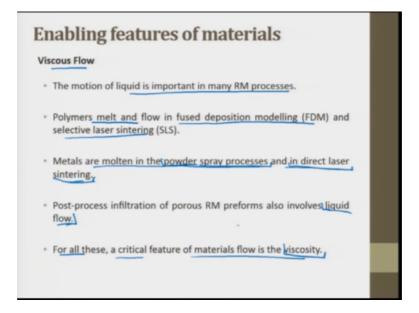
Some enabling features of materials number 1 is viscous flow, the motion of liquid is important in many rapid manufacturing processes because as we said the material has to be melted as a big sometime it is in the filament form some sometime it is in powder form. So, material has to be melted and has to be, then deposited layer by layer to form a final rapid manufacturing build.
