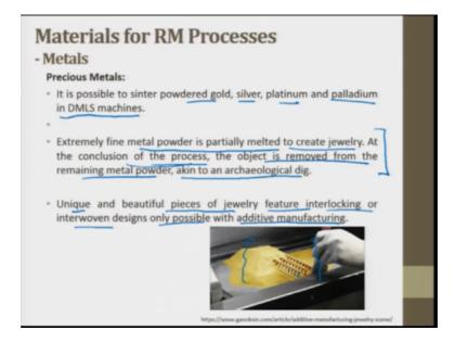
Next is precious metals, it is possible to sinter powdered gold, silver platinum, palladium using direct metal laser sintering machines. Extremely fine metal powder is partially melted to create jewelry. At the conclusion of the process the object is removed from the remaining metal powder akin to an archaeological dig.
