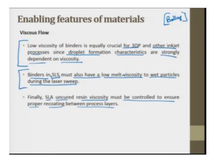
Low viscosity of binders is crucial for 3D printing as well and other inkjet processes. Since droplet formation characteristics are strongly dependent on viscosity. Droplet formation happens in certain processes like 3D printing and there certain defects like balling defects I will discuss about the defects, balling is one of the defect that is the function of viscosity only. What is balling?
