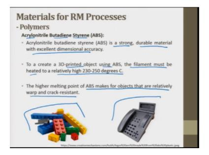
So, let us this try to discuss these polymers ABS PLA and PAV what is ABS? It is a acrylonitrile butadiene styrene. So, this ABS is a strong durable material with excellent dimensional accuracy. To create a 3D printing object using ABS the filament must be heated to a relatively high temperature, I have discussed the difference of ABS and PLA in the demonstration that we had in 3D printing.
