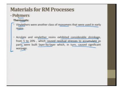
Next is thermosets materials which I have discussed before nylon, PLA, ABS these are polymers these are thermoplastic. Next is a range of thermoset materials such as vinylethers, now vinylether were another class of monomers that were used in early resins. Acrylate and vinyl ether resins exhibited considerable shrinkage from 5 to 20 percent which caused residual stresses to accumulate as parts were built layer by layer which in turn causes significant warpage.
