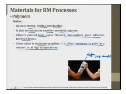
Next is nylon; nylon is a strong flexible and durable material, as you can see here in figure the prosthetic arm is made of nylon and this figure demonstrates that it has high strength. So, they are into arm wrestling, so nylon also demonstrates excellent material memory. Objects printed from nylon filament demonstrate good adhesion between layers, designers and engineers performed test using functional prototypes printed from nylon.
