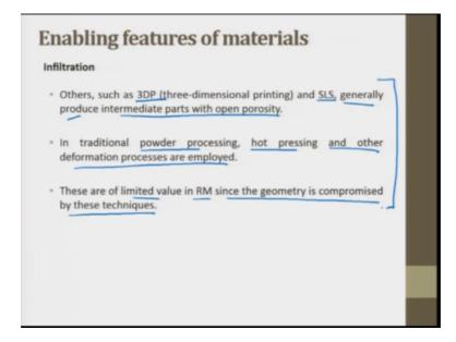
Infiltration others such as 3D printing and SLS generally produce intermediate parts with open porosity. In traditional powder processing hot pressing and other deformation processes are employed. These are of limited value in rapid manufacturing since the geometry is compromised by these techniques. So, high temperature post process sintering is sometimes useful if the kinetics for densification are acceptable and it is one of the criteria.
