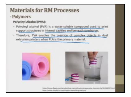
Next is PVA polyvinyl alcohol is a water soluble compound used to print support structures in internal cavities and beneath overhangs, you can see as it is given in the figure this white color PVA. So, it is dissolved in warm water as we showed you the two kind of nozzles were there in the laboratory demonstration one is support material another is the base material.
