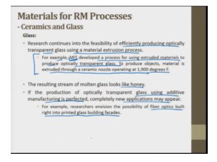
Research continuous into the feasibility of efficiently producing optically transparent glass using a material extrusion process. For example, MIT developed a process for using extruded materials to produce optical transparent glass. To produce objects material is extruded through a ceramic nozzle operating at 1,900 Fahrenheit. So, this is one of the research that is carried out in MIT institute.
