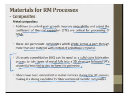
Additives to control grain growth, improve sinterability and adjust the coefficient of thermal expansion are critical for processing of functionally graded materials. These are particulate composites which grade across a part through, more than one material with control of anisotropic response. Ultrasonic Consolidation which is UC can be used as a solid state fabrication process to join layers of metal foils into 3D structure followed by a sequential machining step to form the geometry.
