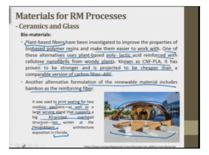
Bio materials, plant based bio fibers have been investigation to improve the properties of bio based polymer resins and make them easier to work with. One of these alternatives use plant based poly lactic acid reinforced with cellulose nanofibrils from woody plants known as CNF PLA. It has proven to be stronger and is projected to be the cheaper than a comparable version of carbon fiber ABS material.
