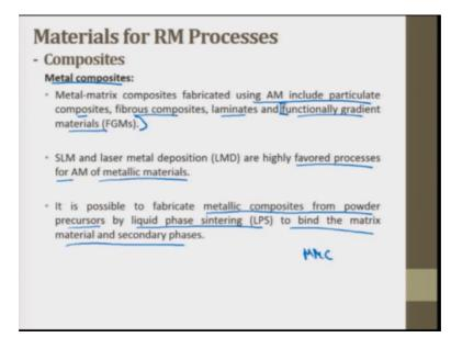
Next is composites, metal composites; metal composites fabricated using additive manufacturing include particulate composites, fibrous composite, laminates functionally gradient materials, FGMs would be taken separately in this lecture. So, SLM and laser metal deposition are highly favored processes for additive manufacturing of metallic materials.
