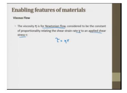
The viscosity eta for Newtonian flow considered to be the constant of proportionality relating to the shear strain gamma to an applied shear stress tau. So, this relation is directly like this then, tau is equal to eta into shear strain. Now many polymers obey a similar non Newtonian power law relationship in which gamma is raised to the power m or less than 1.
