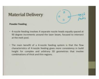
4 nozzle feed involves 4 separate nozzle heads equally spaced at 90 degrees increment around the laser beam, so it is something like this. Focus to interest intersect at the melt pool, these are all nozzle feeding. The main benefit of 4 nozzle feeding system is that the flow characteristics of 4 nozzle feed use more consistency in building height of complex and arbitrary 3D geometries that involve a combination of thick and thin layers.
