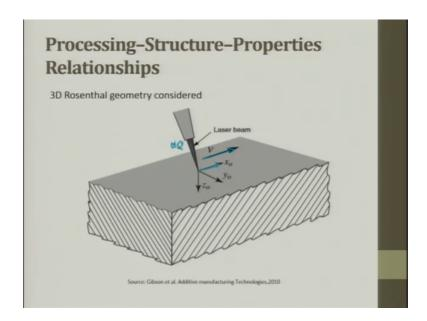
So, Rosenthal geometry is there this is a laser beam it moves at a velocity V. So, at x plane, y plane, z plane here is the alpha and Q heat and the and the thermal conductivity.
