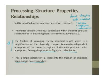
The simplest model material deposition is include ignore, the model considers only heat conduction with the melt pool there is convection and radiation, but we take only conduction and substrate due to the travel heat source moving with a velocity of V.
