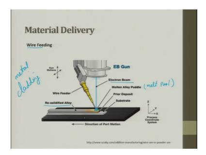
So, wire feed, so this is the wire which is getting fed it looks like your make system and take system. So, this is a wire feeding coming up here is a laser, so this laser or the electron beam, so it comes and hits at the pool and here it melts the here is a melt pool we talk about. So, this is the molten they call it as puddle we will call it as melts pool. So, this is this is the wire coming here electron beam; electron beam can be replaced by laser.
