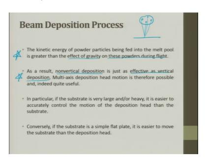
The kinetic energy of the powder particle being fed into the melt pool is greater than the effect of gravity on this powder during flight, understand this point. This is very important. The kinetic energy of the powder particle being fed into the metal pool is greater than the effect of gravity on these powder during flight ok. So, this make sure that it does not there us is a buoyancy which comes because of this buoyancy in the melt pool there is a buoyancy, there is a density difference.
