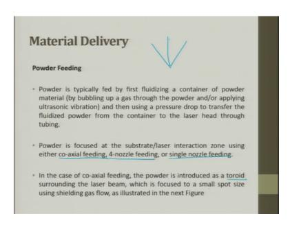
The powder is typically fed by first fluidized fed by first fluidizing a container of powder material and then using a pressure drop to transfer the fluidized powder from the container to the laser head through the tubing. So, when you start flowing the powder it is not necessary the powder should keep flowing because of gravity. So, here you have to create a pressure drop, so that the powder flows properly and it hits at the liquid metal.
