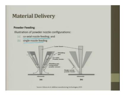
So, you can see a coaxial feed, this is co axial and b is single nozzle, so this is single nozzle. So, you can see here this or shielding gases switch come and here are powders which come powders can be same powder, powders can be alloy powder, so whatever it is you can do is it no issues. So, this is a diagram is talks about coaxial feeding, this is talking about a single axial nozzle feeding.
