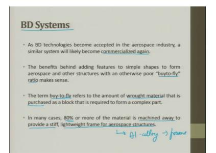
As BD technologies become accepted in the aerospace industry, a similar system will likely become commercialized again. The benefit behind adding features to simple shapes to form to form aerospace and other structures with an otherwise poor buy to fly ratio make sense. So, now, what is happening? Very complex geometry can be easily made through using this lens process or this beam delivery process direct metal.
