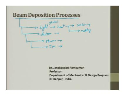
So, the next lecture of discussion in this course of Rapid Manufacturing, we will see the topic on Beam Deposition Processes. So, as it is very clearly says there is a beam. So, this beam can be made of light which can convert into heat, we can use it or we can use electron as a beam and we can do it we can use a plasma as a beam and then we can do it. So, it is nothing, but a source which can be lights, which can be electron source, it can be a plasma source.
