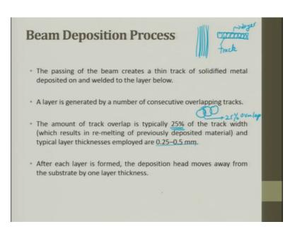
The passing of the beam creates a thin track of solidified metal deposited on and welded to the layer below. A layer is generated by a number of consecutive overlapping tracks ok. So, what your talking about these are the tracks several of these tracks forms a layer, these are the tracks and these are the layers these are tracks and the entire thing is a layer. The amount of track overlap is typically 25 percent, so what are we talking about? One track is typically 25 percent.
