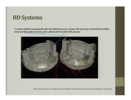
So, this is a metal satellite housing built with the hybrid process is shown, the base was machined from billet stock and the thin walls structures were added with the LENS DED process. So, thin wall structure this is all done by LENS, these are thin wall structures.
