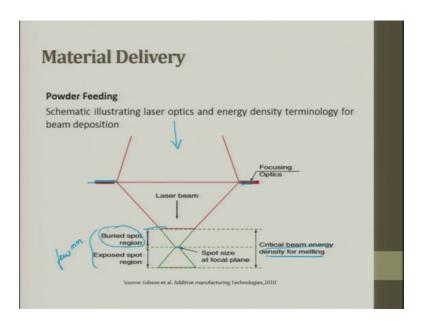
So, this is what we were trying to talk about. So, here as focus optics, so the laser beam comes from here. So, you put an optics; you put an optics, so the optics will they converts. So, here is the, this is the buried spot region, this is the exposed spot region, this is the spot. So, from here to here this is a critical beam energy density for melting
