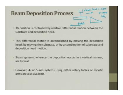
The deposition is controlled by relative differential motion between the substrate and the deposition head. This differential motion is accomplished by moving the deposition head
