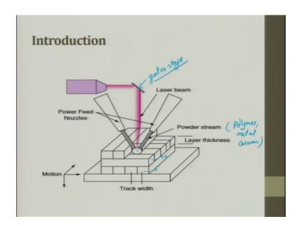
If you look at it, this is a powder feed nozzle. We have to powder feed nozzles, so and then you have a lunch with comes. Suppose you try to take a powder as you can take a polymer powder, you can take a metal powder, you can take a ceramic powder and generally ceramic needs a very high power. So, what will do is we try to have this ceramics which will not melt, but it will the metal will melt and the ceramic gets embedded into the liquid metal and then it forms a composite.
