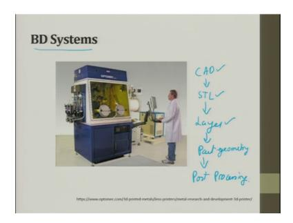
So, here is a typical BD system, so this is how the entire system looks like and you have the CAD is fed here. So, the CAD is come it so CAD, CAD to STL, STL to layer, layer to part, part to post process is done in this machine. So, CAD, STL, layer cutting is done and then it is fed to the machine the part geometry is getting developed in this machine, so where we use metal wire for or wire feeder for doing it.
