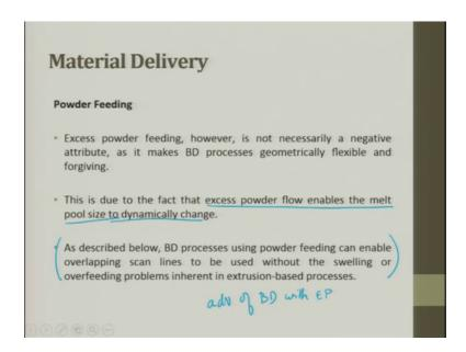
Excess powder feeding; however, is not necessarily a negative attribute, as it makes beam delivery process geometrically flexible and for giving. This is due to the fact that excess powder flow enables the melt pool size to dynamically change. So, excess powder flow dynamically changes the melt pool, when you dynamically change the melt pool you do not know whether you get a larger track or a smaller track.
