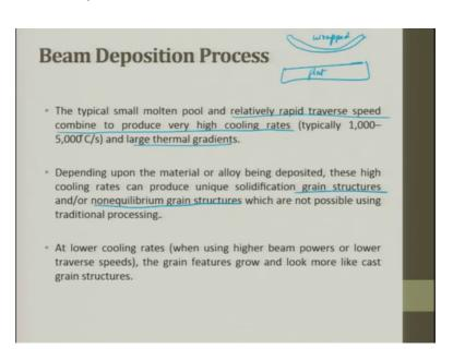
A typical small molten pool and relatively rapid traverse speed combine to produce very high cooling rates and large thermal gradients, rapid traverse speed combine to produce very high cooling rates. So, gradients are created, these gradients are disaster you should try to avoid having large thermal gradients.
