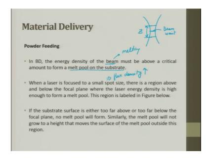
In BD the energy density of the beam must be above a critical amount to form a melt pool on the surface. So, it depends on the laser beam power laser beam because melting, it has to help in melting. When the laser is focused on a small laser spot flux density increases, there is a region above and below the focal plane where the laser energy density is high enough to form a melts pool. This region is labeled in the figure we will see the figure.
