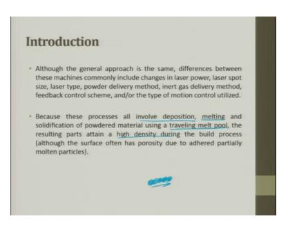
Although the general approach is the same differences between these machines commonly include changes in the laser power, laser spot size, laser type, powder delivery, method inert gas delivery method, feed feedback control scheme and or type of motion control utilized. Motion control is a belt drive lead screw whatever it is.
