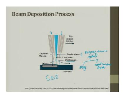
So, the figure clearly says this is a substrate here, it is flat and then you have a deposited material see these deposited materials flow through this these 2 orifices. So, it come at a pressure, so when the particle comes it comes in along the axis it tries to meet and it tries melting at this point, when it starts melting at this point it slowly gets deposited. So, you can have the powder coming from this powders can be polymer again, it can be ceramic, it can be metal.
