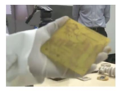
This is printed circuit board. You can see this is the raw PCB, these are the tracks. We have asked a material from the yellow surface area where yellow area here. This is this brown one is copper bead here.
