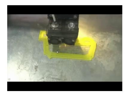
In that case, we will have a support any modern materials you know now this is happening this first layer was brimmed. And after first layer the other layer the second layer is now being manufactured. But is preparing support, you can see it is preparing support here because it was an angle in the component.
