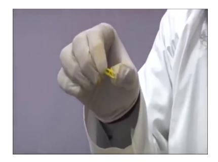
So, these supports you can see this was the final component that was desired here final feature of my component here and this is the support that is removal, so it is hollow from inside. So, this is the product that we have manufactured in our demonstration in rapid prototyping or we also call it additive inspection here. So, this is TECHB V30 machine fused deposition method machine.
