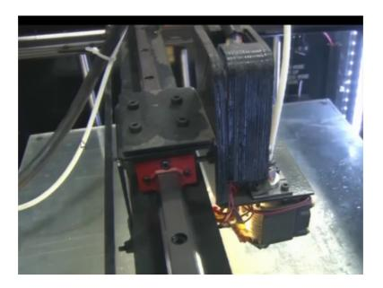
Now, this is our head this is our and there are heaters here that are heating. The filament the spool is coming through this tube the white tube the filament is coming through this y tube ok. So, this is the head that can be moved or this is our x and y movement ok. In z moment that actually bed is moving up and down that movement is controlled with bed and they are two nozzles here. The only one nozzle is active at this point of time.
