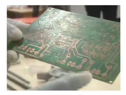
And then we have the chemical coating also to make it green coated at all and the copper tracks are there. And to prevent it from oxidation, we use green coating and green liquid is here to make it free from oxidation with that is a that is green coating is happening.
