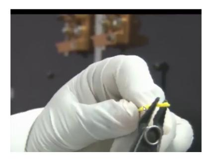
The tip of the filament or the end of the filament is not proper. So, we are going to cut it they have cut it, so it is now flat at the end or screw at the end. So, this is the roller. This would help to take the filament forward when this rotates the filament is carried forward in this direction; upward direction.
