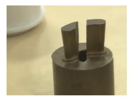
So, there is one more job of brass this profile is called as aerodynamic profile. So, our students at IIT Kanpur of working on this high pressure air this specific component is used to there. So, this kind of job also is carried out with the subtractive method of machining only with meaning machine.
