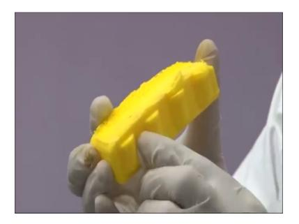
So, this part this support I am removing. So, the brim part is there on the machine only. So, this is the final product that we have manufactured. So, we can see here that on this support that complete material deposit is not it is only the mesh. So, as the minimum material is deposited that can support the main material that is the main filler material that is we used here. So, here as we are using single spool the same material is being used as support and main material.
