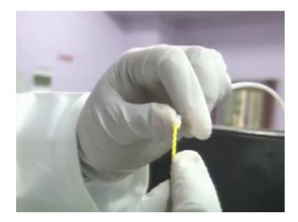
Now, we are entering the filament into the tube that is connected to the PU connector. And this tube is also very much according to the diameter of the filament 1.75 inside diameter 1.75 plus alliance. Alliance is 0.11 0.85 mm in a dia.
