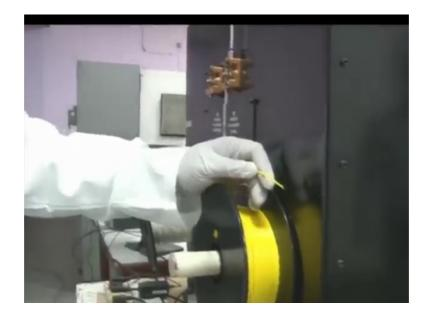
This is again this is the filament of size 1.57 mm. Now we can see that the filament a little is little distorted from the tip that is it would not enter the rollers properly.
