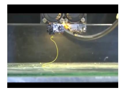
In manual control, so we will we are going to check manually that whether the things are moving. Yes, we have we are checking the material is coming in material is coming out you can see the material is coming out. So, we are manually checking whether the feeder is working or not ok. So, the material is coming out, the up extruder is being checked here for it is proper setting. Again we can see extruder is activated. In this way, we check that everything is quite well or not.
