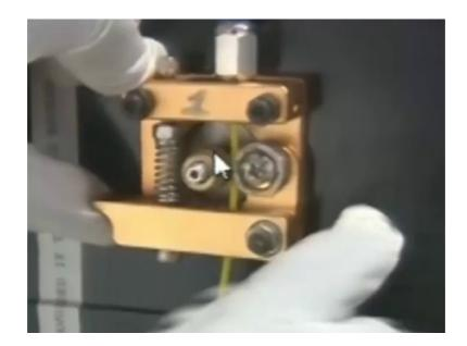
So, this roller that I mentioned that is responsible for feeding; this is also known as feeder. So, we are using this pulley and feeder two rollers. One roller is pulley; another roller is feeder.
