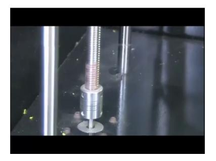
Again you can see the rotation the bed is moving up in a upward direction. Because we do not know what is the thickness of the glass plate that if you put on and also there is there of the fevi stick as well that we have that is there. So, the bed would touch the nozzle end to set the zero value. No yes, it has started the printing.
