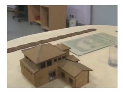
This printing in teak ply, and we print and cut when we assemble. So, this is a printing advisor cutting of wood, this is in teak ply the 3D model is made. Now this is actually a very old technology cut and paste cut and paste there was no 3D printing or the no advanced machines were there. So, this was the way to develop the model.
