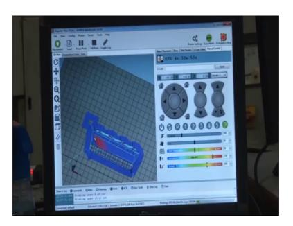
So, what we can see here is the machine is running we can see the simulation of the machine as well as the actual machine is running here. So, the stimulus is happening you will see the material is being deposited here. So, all these layers that you can see as mesh here these are supports.
