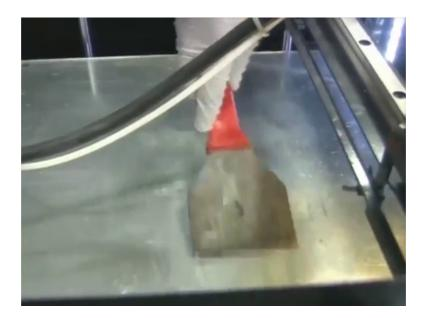
So, some of the liquid cleaner is sprayed and it is cleaned with the help of spatula. So, the whole machine header is actually glass, so we have to be careful. So, what is this white milky carer? White milky material it is nothing, but we have used fevistick that is the adhesive material this fevi stick.
