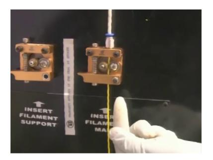
Now, we can see here that how the feeder helps to feed the material this is the feeder; feeder is rotating ok. This is a roller mechanism here pulley and feeder pulley and feeder is there feeder is rotating to feed the material towards the upward direction, but this is not the part of the (Refer Time: 13:50), but this is used for the deposition. So, this is how the machining is happening ok.
