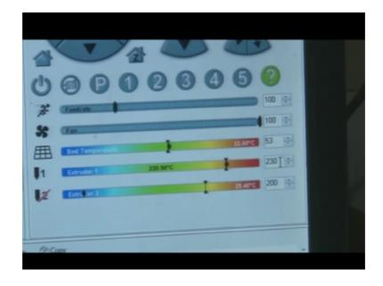
Now, the temperature is actually at 53, 230 degree; yes, the temperature is 230 degree. 230 degrees for the extruder 1, 53.6 degrees is for the bed yes; that means, the as I said 5 degree variation I will have to correct myself this machine is quite precise or sensitive to temperature. So, the temperature 53 degree was set. So, it is within 1 degree 230 it might be 229 or 231, so within 1 degree of the resolution.
