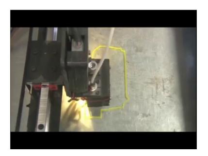
The first layer is started here now. It is now printing, it is minting. This is the brim command that we mentioned before and brim is bring fabricated before actual model. So, this is a very first line that is being drawn by the machine. So, it is running at the speed.
