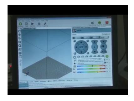
So, the temperature is kind of trying to come to this desired input here to 230 degrees for the nozzle 55 degrees for the bed. It will take about 15 minutes. By the time, we can prepare the bed. So, let us try to start the cleaning and loading and unloading of the material.
