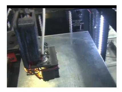
So, let us see how to load and unload the filament. So, this is this black portion this is a PU connector. So, PU connector can be connected, it can be screwed in and out. So, we have unscrewed it ok.
