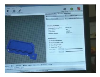
So, this brim is you can see. This cure is here. Why this cure is here? This cure is for holding. We need to hold the job and take it off. It hold the brim; hold the brim layer and take it off ok. This scale is for the holding and the other portion this outer portion is this outer portion is the brim because it has to it would like to save the edges or the make the edges proper brim is only at the edges it had been rough, it would be along all the surface complete surface of the job ok.
