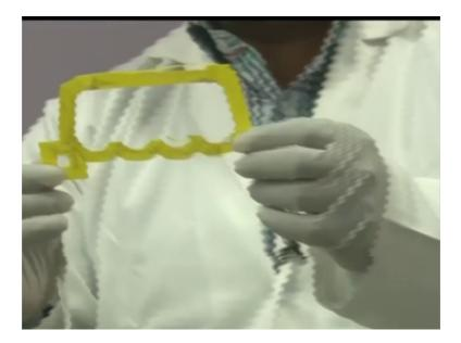
Now, are going to demonstrate this, but we are going to clarify you that this one thing this is brim. So, this is brim that is taken off from the job that is prefabricated. So, this is the model that would be developed. So, this is the pocket; this extra material is brim, this extra material is brim ok. This whole material is brim.
