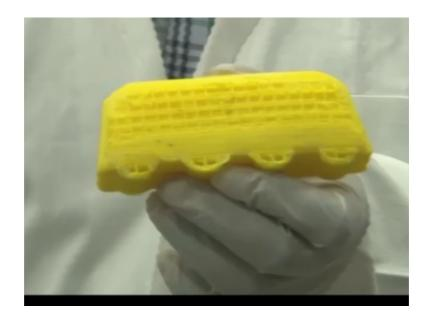
This first here this is actually the brim, this is the model that we have. This is the model that is produced. So, it will deposit the material the little more material. So, this is this material was produced in this way this. So, this extra material is brim, also we have more extra material here those are supports that we will just try to show you how when we remove them.
