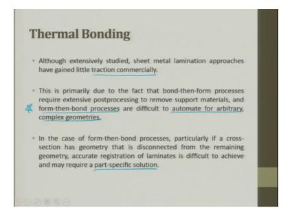
Although extensively studied, sheet metal laminated, lamination approaches have gained little traction commercially, because the final output was not a solid part, which can be a directly taken for rapid manufacturing.
