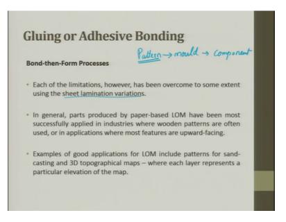
Each of the limitation; however, has been overcome to some extent using a sheet laminate variations. In general, parts produced by paper based LOM have been most successfully applied in industries where would patterns are often used.
