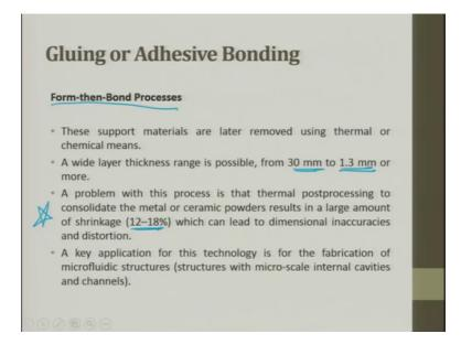
These supporting materials are later removed using thermal and chemical means. the wide layer thickness range is possible from 30 millimeter to 1.3 millimeters it can be done. A problem with this process is that thermal post processing to consolidate the metal or ceramic powder results in a large amount of shrinkage 12 to 18 percent, which can lead to dimensional inaccuracies and distortion.
