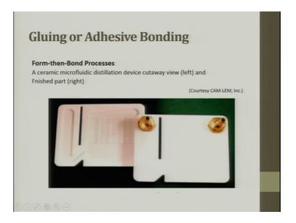
So, a ceramic micro fluidic distillation device cut away view left and the finished product is shown here, so that this can be used for micro fluidic application.
