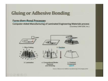
So, this is form then bond, first we use a laser. So, slice cutting is done then what we do is; we try to cut then stacking, then stacking is placing them on above each other.
