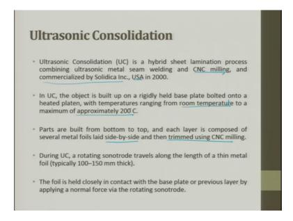
The ultrasonic consolidation is a hybrid sheet lamination process combining ultrasonic metals seam welding and CNC milling. So, metal seam welding and CNC milling and commercialized by Solidica Inc, USA in 2000.
