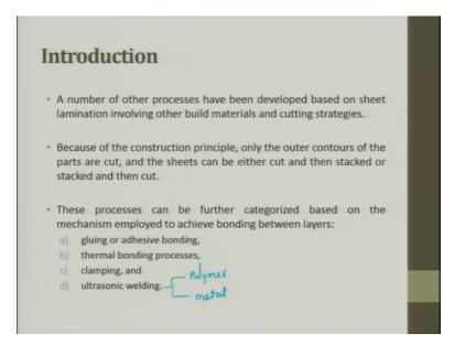
A number of other processes have been developed based on the sheet laminate involving other building material and cutting strategy. So, here we do not you supporting structure, because the supporting structure that sheet whatever is there which is placed. So, you have the sheet and then on wherever there is an extra material required. So, this will be stacking layer by layer by layer and finally, once the object is done, you chill out all the squares and you take the product out.
