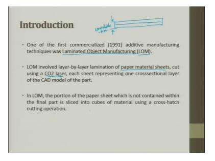
One of the first commercialized additive manufacturing technique was laminated object manufacturing, which is otherwise called as LOM. LOM involves layer by layer lamination of paper material sheet, cut using a CO2 laser, each sheet representing one
