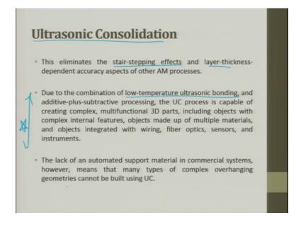
This eliminates the staircase effect, whatever is getting formed when to do layer by layer approach, we have this staircase that is removed by ultrasonic consolidation method and layer thickness depends accuracy aspect of other AM processes.
