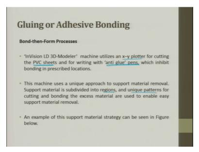
This is a next one; so a small of shift of the regular process in vision LD 3 D Modeler machines utilize a x-y plotter for cutting PVC sheets and for writing way with anti glue pens, which inhibits bonding in prescribed locations. So, PS PVC sheets, anti glue pens are used drop and then you get the information.
