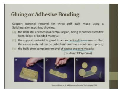
So, you can see, look at it; supporting material removal for three golf balls made using a solid dimension machine, showing. So, the ball still, the ball still encased in a certain region, being separated from the large block of bonded material.
