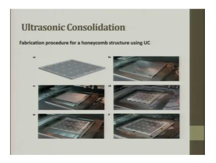
So, this is what it is. So, you have the fabrication procedure for a honeycomb structure using UC. So, honeycomb structure, so this is b. So, you keep, you keep the other layer, then you see that layer which is placed here, then honeycomb, whatever it is we have done here then e and then f. So, ultrasonification happens consolidation happens and then you get the layer.
