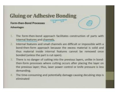
The form then bond approach facilitates construction of parts with internal features and channels ok. The form then bond approach facilitates construction of parts with internal features; that means, to say a egg yo albumin yolk right.
