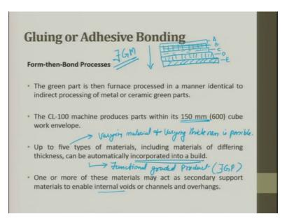
The green part is then furnace processed in a manner identical to indirect processing of metal and ceramic green parts. The CL 100 machine produces part within it is 150 millimeter cube work envelope. Up to five types of material include material of different thickness, can be automatically incorporated into the build.
