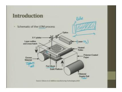
The schematic diagram of the LOM is shown here. So, look at it. So, you have a laser laser comes here, this is a CO2 laser and from here you have optics. This is, from this optics, it goes to a it goes to a galvo. So, from a galvo it is hit on the table. In the table you will have a laminate, you will have a laminate sheet that is what is laminate and here you now, you can think of like every time who is going to plays the sheet.
