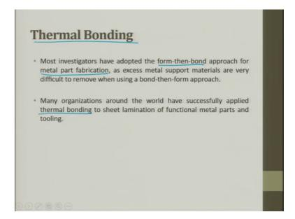
The most investigators have adopted the form then bond approach for metal part fabrication, as excess metal supports materials are very difficult to remove when using a bond, then form approach. Thermal bonding, metal parts, form and then bond approach, three important points.
