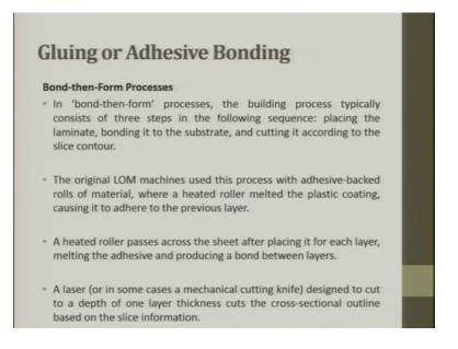
So, bond and then form process, in bond then form process, the building process typically consists of three steps in the following sequence: placing the laminate, bonding it to the substrate where the part is getting developed and cutting it according to the slice contour.
