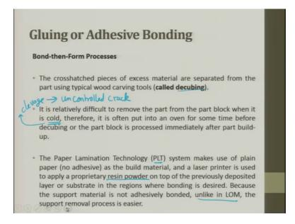
The cross hatched piece of the excess material are separated from the part using typical wood carving tool are called decubing. Straight away trying to break, sisil it out and remove. It is relatively difficult to remove the part from the part block when it is cold, therefore, it is often put into a woven for sometime before decubing or part block is processed immediately after the part building happens.
