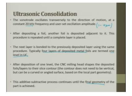
The sonotrode, moment you say ultrasonic with we use 21 kilo hertz. Yes, sonotrode oscillates transversely to the direction of motion, at a constant frequency of 20 kilohertz and the user set oscillation amplitude.
