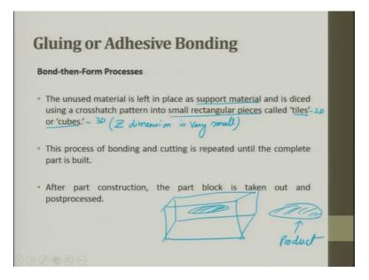
So, bond then form process the unused material is left in place as supporting material. This what I say, there is no supporting structure as we use in fdm process is used here and is diced using a cross hatch pattern into small rectangular pieces called as tiles or cubes. Tile is a 2 D, cube is a 3 D and here the Z dimension is very small ok.
