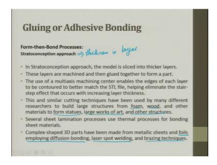
Stratoconception approach, in stratoconception approach, the model is sliced into thicker layers. These layers are machined and then glue together to form a part. For example, you take a bread loaf, take individual bread slice, this bread slice thickness is there, cut whatever information you want in each slice, than stack it together, the layers are machined and then glue together to form a part.
