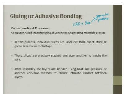
Computer aided manufacturing of laminated engineering material process; in this process individual sizes are laser cut from sheet stock of green ceramic or metal tape. These slices are precisely start to one over each, this is what I said is a limitation.
