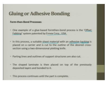
One example of the glue based form, then bond process is the 'Offset Fabbing' system pattern by Ennex Corp, USA. In this process, a suitable sheet material with an adhesive backing, a suitable sheet material with adhesive backing is placed on a career and is cut to the outline of the desired cross section using two dimensional plotting knife.
