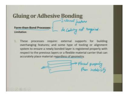
So, that is the advantage of form. So, form has internal features, internal features and decubing not required. The limitation is these process is required external support for building overhanging features; but this was not there in the LOM process and some type of tooling or alignment system to ensure a newly bonded layer is registered properly with respect to the previous layers or a flexible material career that can accurately be placed material regardless of the geometry.
