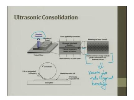
So, this is what is the rotating sonotrode; so here if you see, this is a heated base, this is how the object is getting built, and here is a rotating sonotrode, it is a drum, which goes from this to this.
