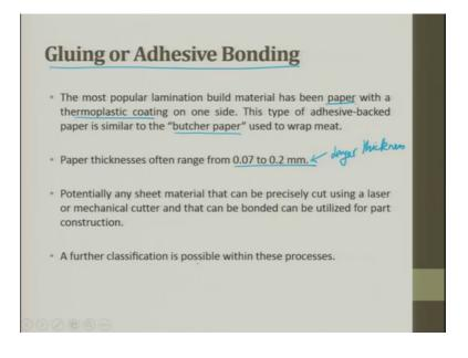
Gluing or adhesive bonding the most popular lamination build material has been the paper with a thermoplastic coating, this is what I said lamination, which you do for certificates paper, with a thermoplastic coating on one side. This type of adhesive backed paper is similar to the butchers paper used in wrapping meet.
