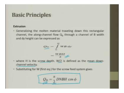
So, Q D the generalized molten material traveling down this rectangular channel the along channel flow Q D through the channel of B with and dy is the height can be expressed in integrating from 0 to H WB dy. So, which is nothing, but W into B into H by 2, where H is the screw depth. W by 2 is defined as the mean down channel velocity, substituting back in the Q D you get this equation.
