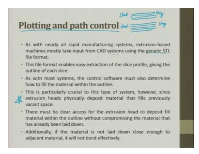
So, plotting and the path control so a path control is start stop this is start stop. So, how do we do it and then how do we come back? Serpentine pattern or we just go like this, this is start this is stop, so these are some of the patterns plotting and path control. As with lean as with nearly all rapid manufacturing system, extrusion based machines mostly take input from the cad system using generic STL file format.
