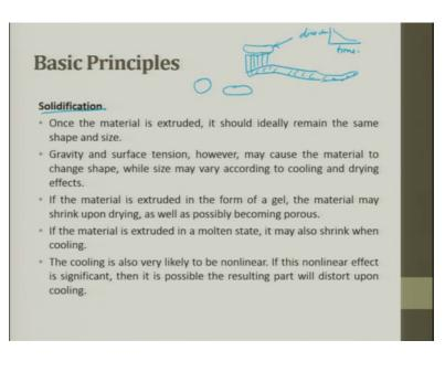
The next one is going to be till now hopper flowing we saw, next one is solidification why solidification? It will lead to delamination you want to avoid delamination, so we have to focus on solidification. Once the material is excluded, it should ideally remind the same shape and size.
