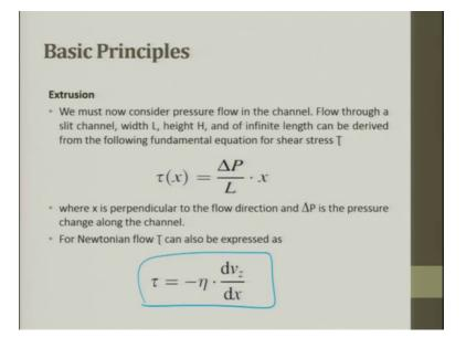
We must now consider pressure flow in the channel. Flow through a slit channel width of L, height is H and the in and infinite length can be derived from the following fundamental equation of shear stress tau; tau is nothing, but d P by L ok. Where x is the perpendicular to the flow direction and d P is the pressure change pressure drop along the along the diameter and L is the length. So, for a Newtonian fluid it is defined like this. So, it is minus viscosity eta into dv z by dx.
