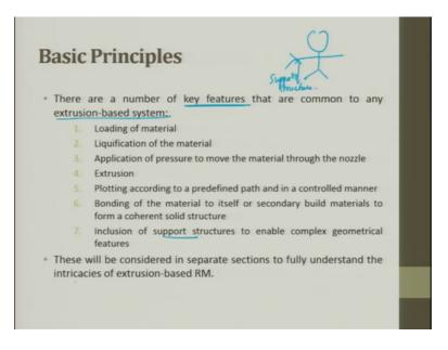
So, there are number of key features that are common to any extrusion based process loading of material, liquefaction of material, application of pressure, extrusion plotting according to the predefined path in a controlled manner, bonding of material to itself or a secondary build material to form a coherent solid structure, inclusion of supporting structure to enable complex geometry features.
