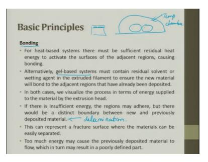
The next key feature is the bonding, as I told you delamination will come. For heat based system there must be sufficient residual heat energy to activate the surface of the adjacent region causing bonding. So, you have one, you have two, so you maintain it under a temperature. This is a chamber temperature chamber so, there sufficient enough to activate and bond.
