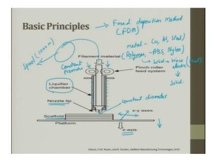
So, this is a basic principle for FDM process Fused Deposition Method FDM process. So, here we try to take a filament wire which is polymer generally, what we uses is ABS; ABS nylon can be used. So, people are now working on various systems you can also have biocompatible material ABS is also biocompatible ABS is there industrial abs is there you can choose any of them choose a polymer.
