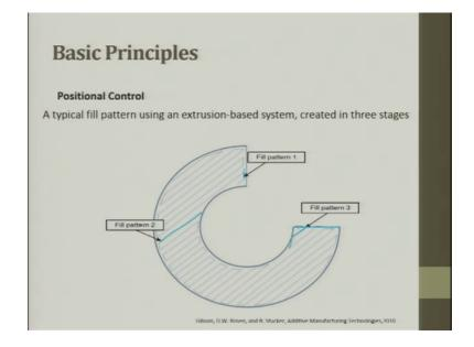
A typical fill pattern can be seen so, this is the; this is the external feature and this is the fill internal fill. So, we can see here this is a pattern; this is a pattern and this is a pattern this top one is a pattern. A position control a typical fill pattern using and extrusion based system created in three stages; one is filling vertical ok, the other one fill pattern is at an angle and the third one is along the a different angle. So, this is the along a straight line.
