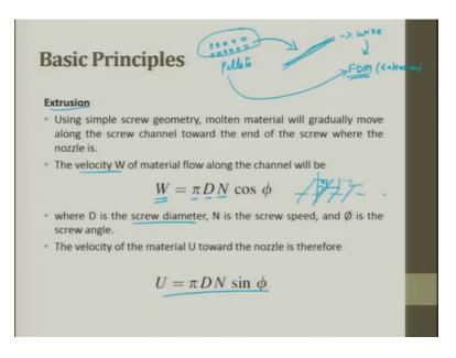
So, the wall thickness that are at least twice the nominal diameter of the extruded nozzle used. So, when we talk about extrusion using a simple screw geometry, molten material will gradually move along the screw this is for injection molding channel towards the end of the screw where the nozzle is velocity W of the material flow along the channel is given as W is nothing, but pi into D into N.
