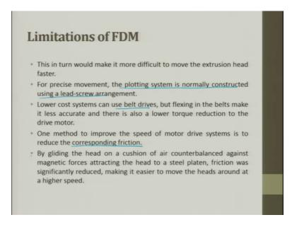
This in turn would make it more difficult to move the extrusion head faster. For precious movement, the plotting system is normally constructed using lead screw this is what I told you. The low cost system will always have built because here the accuracy is are not there.
