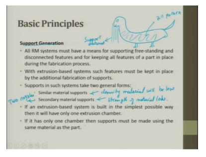
Support generation this I was trying to tell you; you have a free hanging surface, this free hanging surface has to be supported. For example, if you want to make, an object like this so this fellow has to be supported from here, this is called as supporting material which will not be the same as you original material.
