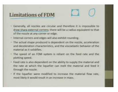
So, the limitation of FDSM generally, all nozzles are circular and therefore, it is impossible to draw sharp external corners, so, we cannot get a nozzle orifice like this, we always get orifice like this. So, these are dead centers where in which the flow will not happened, so we do not go for square nozzles
