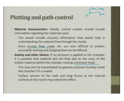
The material characteristics I have told you in the plenty, this would include viscosity information that would help in understanding the material flow through the nozzle. Since viscous flow, creep etcetera are very difficult to predict accurate starting and stopping flow can be very difficult.
