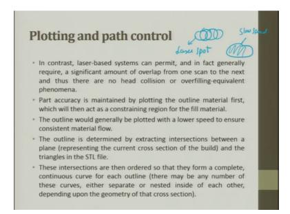
In contrast, laser base system can permit and in fact generally require a significant amount of overlap from one scan to the next and thus there are no head collusion or overfilling equivalent phenomena. One spot the other spot this is a laser spot.
