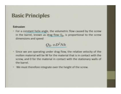
So, the extrusion for a constant helical angle, the volumetric flow causes caused by the screw in the barrel known as a drug flow Q D is proportional to the screw dimension and this speed.
