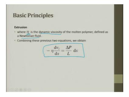
So, where d where eta is nothing, but the dynamic viscosity of the molten flow defined by the Newtonian fluid. Combining these previous two equations we have this is the final equation from here you can try to find out the eta value and try to substituted in the equation.
