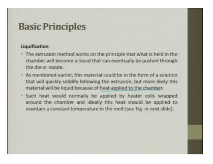
Liquefaction, the extrusion method works on the principle that what is held in the chamber will become a liquid that can eventually be pushed throw a die or a nozzle. As mentioned earlier this material could be in the form of a solution that will quickly solidify following the extrusion, but more likely this material will be a liquid because of heat applied to the chamber.
