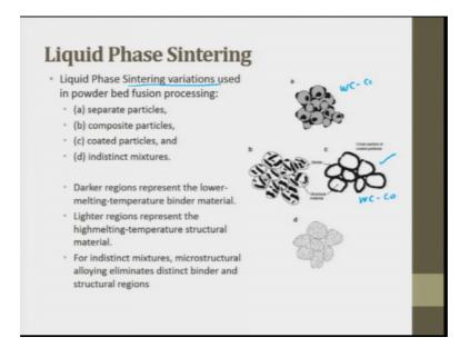
So, the liquid phase sintering variations used in powder bed fusion processes are; a, is separate particles these are all sintering variations separate particles. Then b is composed particles these are composed particles c, are coated section these are all coating particles d, is indistinct mixture so you have all the four. Darker region represents the lower melting point of binding temperature these are all darker lower.
