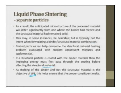
As a result the anticipated microstructure of the processed material will differ significantly; from one where the binder had melted and structural material had reminded solid. Completely different phenomena can happen; this may in some instance be desirable, but it typically not the intent when formulating a binder slash structural
