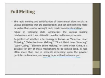
The rapid melting and solidification of these metal alloys results in unique properties that are distinct from and can sometimes be more desirable than caste or wrought parts made from the identical alloys. In the next slide we will saw the summary; the various binding mechanism which are utilized in powder bed fusion process.
