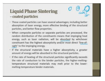
The coating the next phase; so first was you had some particles little little bit here and there then inside the particle you had a binder material. Now the third thing is I am trying to give a coating on top of the powder particles ok. This is the third type of in liquid; how are we preparing the particles for liquid phase sintering these coated particles can have several advantages including better absorption of laser energy because this will can absorb.
