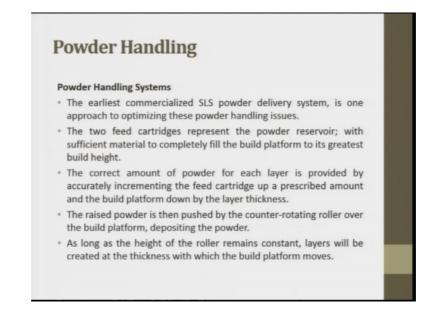
The earliest commercial commercialized SLS powder delivery system is one approach to optimize this powder handling issues; to feed cartridge presents the powder reservoir with sufficient material to completely fill the build platform to it is greatest build height so it was taken care.
