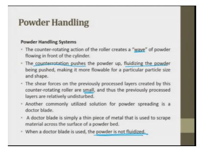
The counter rotating action of the roller creates a wave, wavy of the powder flowing in front of the cylinder. So, this wave has to be made flatten because when the next layer laser curing is happening or laser sintering is happening this undulation on the surface reflects it so we have to be very careful.
