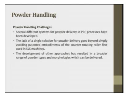
Powder handling challenges these powders are not so easy to handle. Several different systems of powder delivery in powder bed fusion processes have been developed. The lack of single solution for powder delivery goes beyond simply avoiding patented embodiments of the counter rotating roller first used in SLS machine. The development of other approaches has resulted in a broader range of powder type and morphologies which can be delivered.
