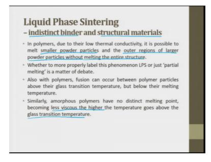
So, the last part of the powder is indistinct binder and structural material. In polymers due to their low thermal conductivity polymers it is possible to melt a smaller powder particles and the outer region of larger powder particles without melting the entire structure. So, sintering; sintering is not melting by the way.
