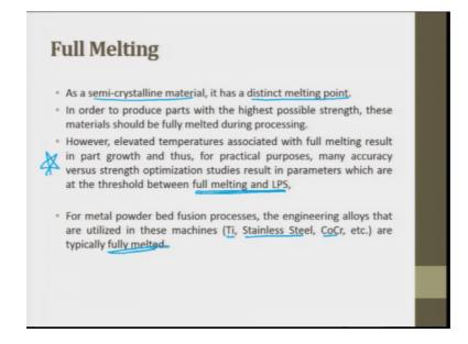
As a semi crystalline material it has a distinct melting point. Crystalline materials it have a distinct melting point amorphous material do not have semi crystalline has somewhere in between. In order to produce parts with the highest possible strength this material should be fully melted during the processing.
