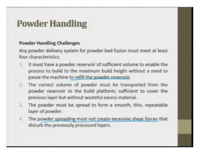
Any powder delivery system for powder bed fusion must meet at least four characteristics. It must have a powder reservoir of sufficient volume to enable the process to build to the maximum build height without a need to pause the machine to refill the powder reservoir. So, this is this is one thing which you have in between you cannot stop. If you stop it refill it and restart it then there will be a delamination.
