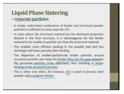
Separate particles; a simple well mixed combination of binder and structural powder particles is sufficient in many cases of LPS. In case where the structural material has the dominant property, desired in the final structure it is advantages for the binder material to be smaller in particle size than the structural material. That means, to say the tungsten carbide only tungsten carbide you would like to have, but cobalt is needed as the binder.
