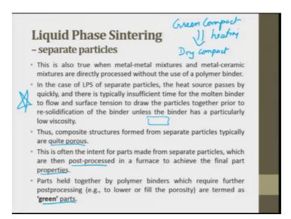
This is also true and metal matrix mixture and the metal ceramic mixture are directly processed without the use of a polymer binder. In this case of LPS of separate particles the heat source passes by quickly. And there is a typical insufficient time for the molten binder to flow and surface tension to draw the particles together prior to re solidification of the binder unless the binder has a particular low viscosity very very important point.
