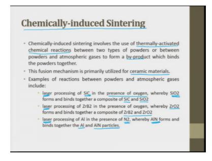
Chemically induced sintering; involves the use of thermally activated chemical reactions between two types of powder or between the powder and the atmospheric gas; to form a byproduct which binds the product together in a very very simple fashion. Such that; you can understand when we make laddu we add ghee to it the function of the ghee is to make sure that this smaller smaller particles are held together right; so here there is no chemical reaction.
