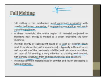
The last one is full melting; full melting is the mechanism most commonly associated with powder bed fusion process of engineering metal alloys and semi crystalline polymers. Most commonly associated with the powder bed fusion processing of engineering metal alloys and semi crystalline polymers.
