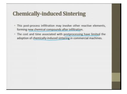
This post processing infiltration may involve other reactive elements forming a new chemical compound after the infiltration. what I was talking is; very high pressure the infiltration is pushing the liquid inside the pores. At some point of time this liquid also
