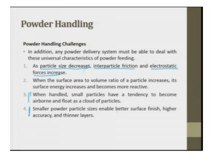
In addition any powder delivery system must be able to deal with these universal characteristics of powder feeding. As particle size decreases inter particle friction and electrostatic forces increases. So, that is why you have agglomeration particle size decreases inter particle friction and electrostatic force increases when the surface area to volume ratio of the particle increases.
