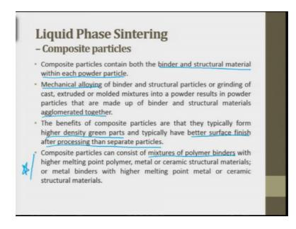
Composite particles the composite particles contain both the binder and the structural material within each powder particle. Composite; let us see the figure composite, so you can see here. Composite b is composite so these are binders, which are inside the particles. Mechanical alloying of binder and structural particles are grinding of caste extruded or molded mixture into a powder results in the powder particles that are made up of binder and structural material agglomeration together.
