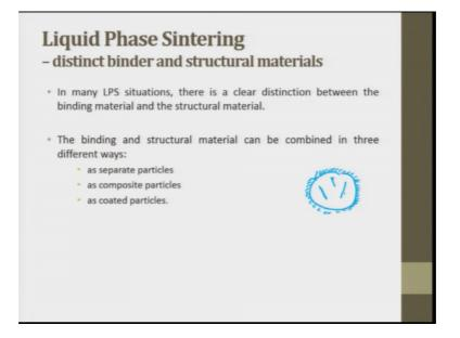
So, liquid phase sintering distinct binder and structural materials in many LPS liquid phase sintering situations. There is a clear distinction between the binding material and the structural material these are binding material very clear distinction was there very clear distinction was there.
