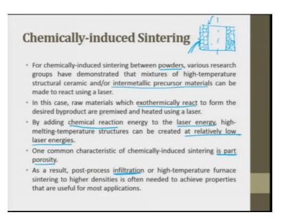
For chemically induced sintering between powder various research groups have demonstrated the mixture of high temperature structural ceramics and intermetallic precursor materials; that can be made to react using laser. In this case raw materials which exothermically react; raw material which exothermically exothermical heat is released while the reaction happened heat is released.
