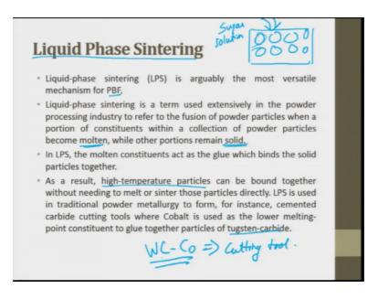
So, liquid phase sintering; so, the liquid phase sintering is arguably the most versatile mechanism in powder bed forming. Liquid phase sintering is a term used extensively in the powder processing industry to refer to the fusion of powder particles when a portion of the constituents within a collection of powder particles becomes molten while other portion remind solid.
