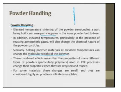
Powder recycling which is one of the biggest things. So, moment you use powder for putting it in the development chamber or in the developing table the two sides the cartridges will have the fresh powder and in the centre what we do is the fresh powder is spread and it is cured.
