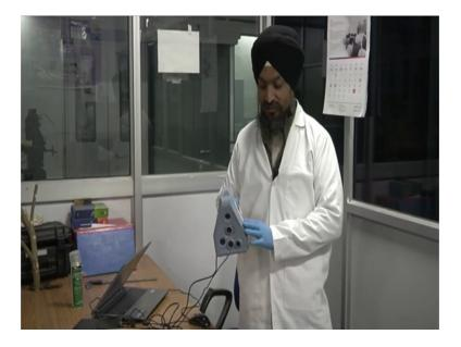
As this is actually hand held 3D scanner which we will discuss in detail and we will see how do we scan this specimen that is made this specimen has various profiles in it. So, this is a blue light hand held 3D scanner. Also we will have a chamber 3D scanner. Picza is the company that is the make of this 3D scanner. This is blue light and that is a red light 3D scanners, we will see the demonstration of this.
