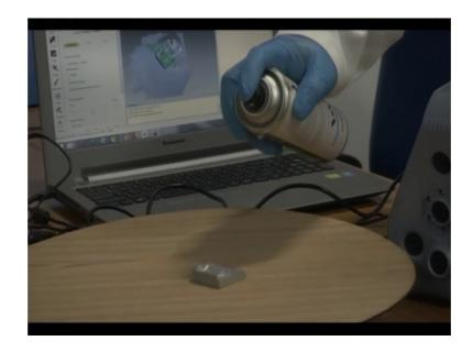
So, we use this developer. This is a liquid spray. So, this can has gas and powder in it. This is of a milky white color when we spray it, you can see it is developing a coating over the object. When this solidifies, it will be white. So, it has made a white thin coating of port powder here this is W1 OO3 developer.
