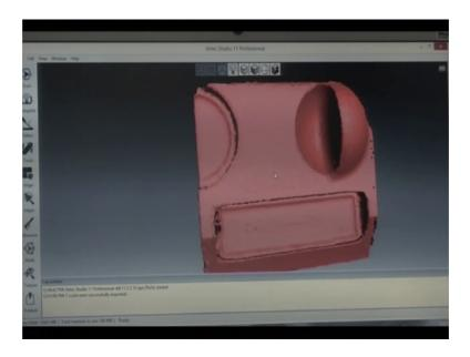
Now, this is the object that we have obtained after the complete scanning. You can see the different views of this you can learn this is this is point view point cloud, this is point cloud, this is the point data or the different point that we have found to, this point cloud helps to get the mesh and that mesh helps to develop is solid model. You can see there is a small flow here this data is not captured, but we will work what we can worked to get this corrected.
