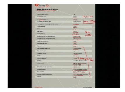
These are the specifications of this scanner that we are going to demonstrate in this lecture. Resolution is 0.21 and accuracy is 0.05, the difference between resolution and accuracy, this is engine metrology. Resolution is the minimum steps taken that we can take forward that is the first step is 0.1, second step can be 0.2 third step can be 0.3 and so on. Accuracy is closest to the results.
