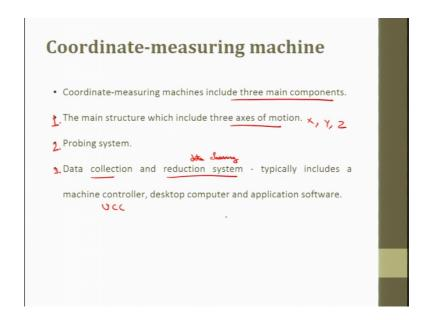
So, coordinate measuring machine include three major components. Number 1 is the main structure with include three axis of motion X, Y and Z-axis. Number 2 is the probing system as I said we have a mechanical probing system here. Number 3 is the data collection and reduction system. Data collection data reduction means we clean the
