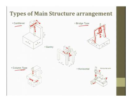
Types of main structure arrangement in the CMM machine are cantilever, you know this is the cantilever beam ok. The cantilever moving beam is moving in X direction. Cantilever beam can move in X direction and all these cantilever beam we have this arm that can move in Z direction. So, second one is column type in column type, we have the table that can move here. This table can move in X and Y direction; in Z direction this arm can move ok. So, this is the column that is attached here.
