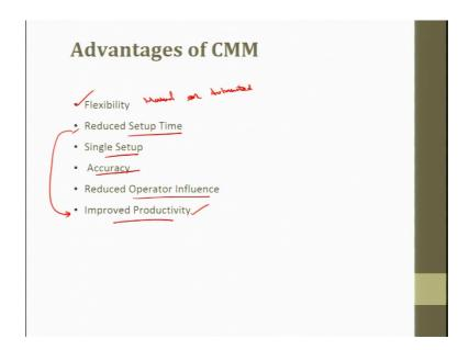
So, advantages of CMM, this I should have told you after completion of the whole lecture ok, but advantages here are the flexibility. Flexibility means we can use it manual or automated ok. So, in manual system, this is a big flexibility that whatever we need to
