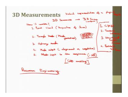
3D measurements, what are 3D measurements, 3D measurement is a process of creating measurement or virtual 3D representation of a physical object. This is virtual representation of a physical object ok. Now, 3D scanners are optical devices used to create 3D measurements or a 3D scanners, we have 3D scanners ok. 3D scans if I say 3D scanners, the outputs are known as 3D scans, 3D scan is the output ok.
