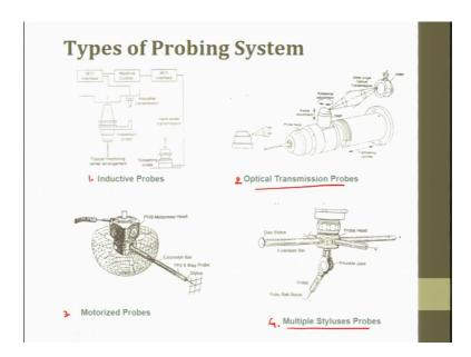
So, different types of probing systems are there, we have inductive probing system like we have inductive probing system, we have machining center arrangements. So, inductive or inductive transmission is the principle in using this probe. Then optical transmission probes are there. When optical transmission is the principal, similarly we have motorized probes motorized probes in which this is just we have the motors and motors can just rotate the probe or move the probe.
