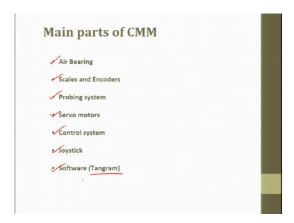
So, main parts of CMM are air bearing, I will show this parts do there. So, we have pneumatic bearings here; so, then scales and encoders, probing system, servo motors, which are just making the parts to move. So, control system is here, joystick is here, software is here, software that we use that is Tangram software.
