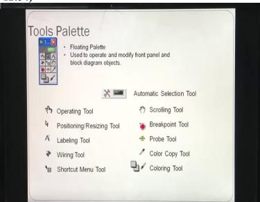
So, these are tools palettes, so there are different types of tool palettes I already discussed about that. So, these are the symbols which is show here like operating tool, positioning, resizing tool, levelling tool, wiring tools, shortcut menu, scrolling tool, breakpoint tool, probe tool, colour copy tool and colouring tool ok. (Refer Slide Time: 13:02)
