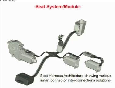
This again is a mechatronics system for the seat module you how much reclining has to happen from the how much seat-forward or seat backward has to happen based on the percentage size in the car is a very important question. So, you again comprise electronic management system which would actually automatically as the passenger comes in there are certain cars where the seat would automatically managed or even at the press of a button it will manage.
