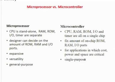
So, essential difference between both is that in a microprocessor the CPU standalone, RAM, ROM, I/O and timers are separate and a design like I decide on the amount of ROM, RAM that
