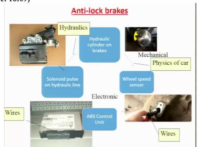
If we looked at what are the different parts or to treat it with different systems which can control this you know differential braking mechanism. So, you have hydraulic assisted braking which is
