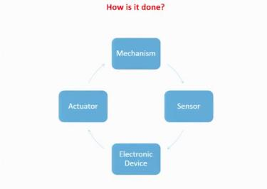
So, how is it done how is mechatronics practiced or how is you know intelligence put into all the products. So, you know you have various components of the system so you have a mechanism in place which is more like the mechanical part of the system of the component. You also have you know an actuator which drives this mechanism. So, this is really the power input and this is really the power output okay of the system.
