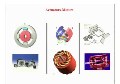
If you look at discretely what these actuators would do these are for example some of the actuators this is a motor where essentially what is happening is that the magnetic field is being varied between different places from 1 2 3 or 4 ok. So, there is a rotating magnetic field of the stator which makes the rotor move which gives you rotar power out of the system these are some of the systems ok and eventually.
