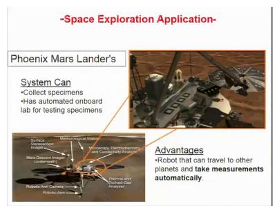
Again what can be done in space this right here is a Phoenix Mars Lander it is a pod which can collect specimens you know through electro microscopy electro chemistry various different analysis on the same pod. So, it is extremely complicated again mechatronics system mechatronic assisted system which we take a sample analyzed the sample send the data. Do all this intelligently while moving itself through a very complex terrain ok.
