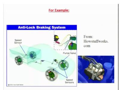
For example if you look at anti-lock braking system in a car so the system basically has a mechanical component which is being pressurized through oil pressure which is controlled through a set of pumps and valves. Pumps are again controlled through motors ok the idea here is that the distribution of the braking force has been you know monitored and accordingly switch braking is provided mechanically to the four different wheels both front and back.
