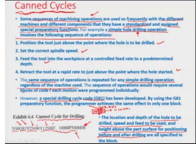
I would also like to now come to a certain different aspect which is about canned cycles. Now one must understand that the whole drilling cycle what we did in the last you know few slides can be represented as one unit or one command okay. So, every time there is a drilling operation you need not go to the different aspects of okay take the drill at a certain position you know dive into the workpiece by having a Z negative value up to a certain extent and then come out of the workpiece okay.
