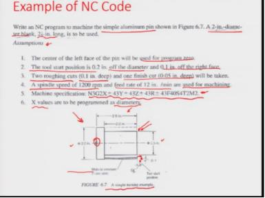
So, let us look at this one example problem here which describes the machining of a simple aluminum pin with a certain head as you can see in this figure right here. it is a simple turning example and here some specifications are given as to what would be the final dimension of the pin which we want to program and a 2 inches diameter blank is carried out or used for formulating the pin which has a head dia of 2 inches.
