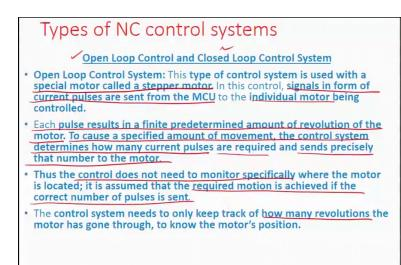
When we go into understanding the programming aspects a little bit of understanding for what all systems are available within any machines are very important. One of the very important aspects behind NC machine is the type of control that has. And we can classify such control as either open loop control or closed loop control. And as the name indicates the open loop control is really without any feedback signal.
