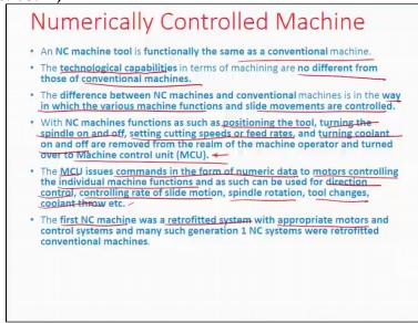
So, when we talk about NC machine tools they are functionally same as convention machines of course in terms of technological capabilities you do not really find many differences from conventional machines only difference between NC machine and convention machine is that there is a difference in way in which various machine functions and slight movements are controlled.
