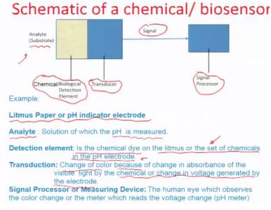
Detector typically does a transduction in terms of the chemical signal being converted into another machine readable signal which can be electrical or optical and the signals are sent in to a signal processor which is able to interpret based on the nature of the signal and that way one can understand the analyte better in terms of its chemical or molecular composition. I explained this how a litmus paper or a pH indicator can serve as a sensor.
