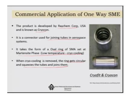
Now, what are the commercial applications of this you know effect, first effect actually came from you know one of the aircraft applications in by Raychem Corporation and this is known as Cryocon. So, what they have done in this case is that this is used for joining tubes in aerospace systems. So, initially the shape will be oval ring of SMA and that will be set at the Martensite phase oval ring ok.
