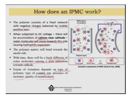
So, how does an IPMC work well first of all it consists of a fixed network with negative charges and that is coming, because of the presence of the sulfonate groups that I we are showing here, and it is balanced by mobile positive ions. So, whenever I am subjecting this system to DC voltage ok I am generating a voltage, what will happen is that, there will be this cations these are the mobile positive ions which will go towards the cathode.
