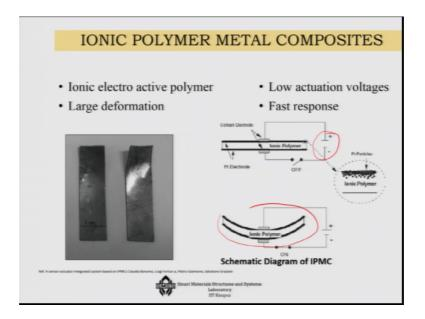
So, this is how then IPMC system works and, if you look at a IPMC composite, then you can see that you know in this particular IPMC system for example, that as I am applying the voltage in this system ok, how these bending is taking place in the system and this is in reality you know how you will be getting it in a same Nafion or Nafion of this type of similar IPMC systems.
