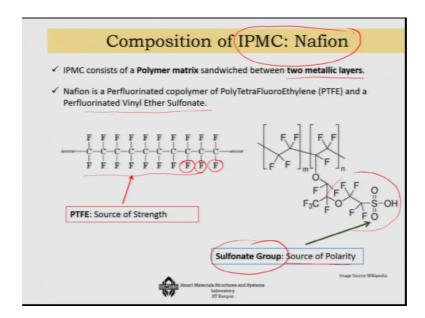
Now, if I focus on one of the most important you know ionic polymer which is known as Nafion, then you would see that it is having actually you know a polymer matrix which is sandwiched between two metallic layers ok.
