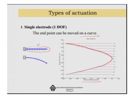
So, if you look at one of the applications like single electrode you know flexible manipulator. So, in this case what you have is that you have a cantilever beam and you apply the voltage, accordingly you will see the tip point getting displaced ok. So, depending on the direction of the voltage, in this case you will see the reversible changes and as a result you will see.
