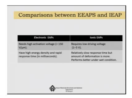
So, if you look at the comparison between the two, electronic activation of course needs a higher actuation voltage, but here you need a low driving voltage, but here the energy density is high and rapid response time.
