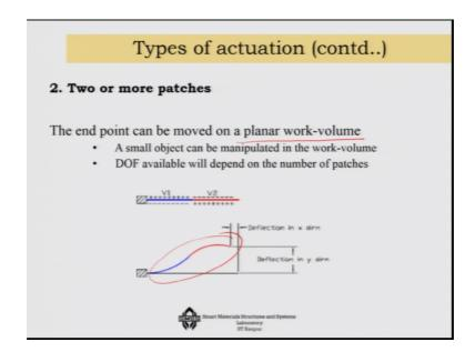
Now, we would like to talk about some of the other you know actuations like, what if I use two or more patches. Well two patches I had already shown you that you can develop a bidirectional deflection in a two patch system and, this can be then used for a planar work volume generation. So, that is something in which you can use this strategy of that selemion with gold and dodite.
