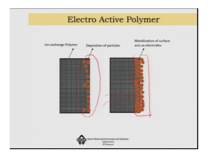
Now, if you look at a one of the most popular electroactive polymers, which is I told you the IPMCs, then it works like ion exchange polymer and if you have deposition of particles here ok, you can actually make a metallization of them. So, you can make a polymer in such a manner that it is partially metalized ok. So, this kind of a thing will actually help to develop cathode or anodic terminals in a polymer.
