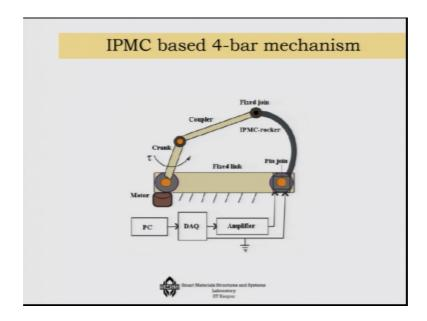
Another interesting thing that can be done is if you develop a 4 bar system in which one of the link is actually flexible. So, then what you can do is that you can use it as a manipulator. So, this is a crank side this is a coupler and this part, if you can change the length of it you can actually use it in terms of developing various different work surfaces.
