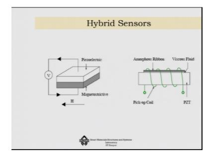
There are many other uses like material which is by more partly piezoelectric partly magnetostrictive, you know amorphous ribbons with viscous fluid in it on a piezoelectric beam so, you can produce many such hybrid effects by using both of them. So, this is where we would like to put an end.
