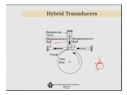
So, that way you can actually detect cracks in the pipeline. Now, you can also develop another intelligent application of the system, which is known as hybrid transducers for hybrid transducers what we have is we have a magnetostrictive rods we know that is a horizontal part and we have piezoelectric stack which is vertical.
