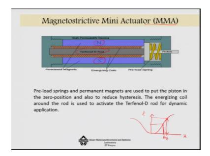
So, these are two ways and in terms of actuators there is one actuator which is very common it is known as magnetostrictive mini actuator. So, what you do here is that you have a Terfenol D rod here and, then you actually have the energizing soils here. So, the coils basically give the magnetic field. Also you give a bias magnetic field, as I told you that this bias magnetic field allows it so, if you still remember H versus the magnetostriction plot let us say you remember that butterfly curve.
