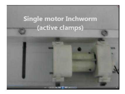
And you know that is happening in a sequential phase, one is touching one is opening up. So, clamping de clamping and the whole system is having a forward motion. So, that is something that you will find in this type of a system.
