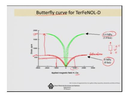
So, what does this butterfly curve means, if I consider the smaller one where it is not compressed, you look at it that if I apply positive load and stress it, I am going to get positive strain in the system. So; that means, if you take a small sample of the Terfenol D rod and, if you apply tensile force you are going to get tensile strain which is fine you know it happens.
