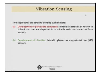
Now, there are two ways I will show you. So, one I told you for the actuator for sensing applications either you can develop you know particulate composites. So, Terfenol D particles are mixed, in a suitable resin system and cured to develop a sensor, or you can develop actually a thin films like metallic glasses as magnetostrictive you know sensors.
