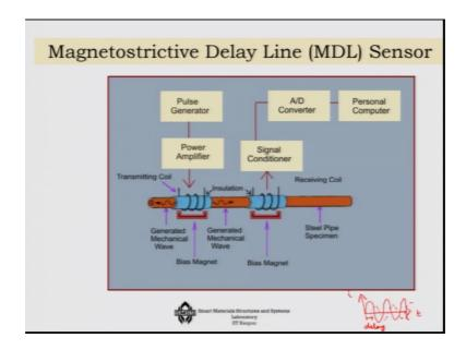
One interesting application is in terms of pipeline sensing, it is also known as magnetostrictive delay line sensor. So, what you have here is that once again you have these you know coils here and, this is a transmission coil and you have a receiving coil at the other point. So, as you are applying an electromagnetic field, what is going to happen is that a vibration is happening and that vibration mechanical vibration is travelling along the pipe.
