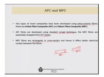
So, we have seen that how we can actually model our magnetostrictive mini actuator. Similar things can be done on active fibers composite and MFCs, but these are consisting of piezoceramic fibers. Now, this AFC fibers are developed using standard sol gel technique whereas, MFC fibers are essentially chopped form of the PZT blocks. So, MFC fibers are rectangular in cross section and that offers you know better contact between the fibers ok.
