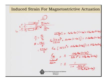
Now, how do we model the induced strain actuation? let us try to work it out we have done it earlier also, so let us consider that we have a beam system like this. So, we have a beam on that beam I have fixed this magnetostrictive mini actuator for the time being let us also neglect the shear lag effect this you know anyway once you know the basic relationships how to add the shear lag effect.
