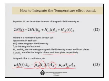
Now if you consider this equation itself then the f is can be replaced by these n which is the number of turns in each coil times i t. And this actually is divided by the length of the coil and that you can take into account here. So, that is for the magnetostrictive material and these two are for the end plates that you have rear and the front plate in our system.
