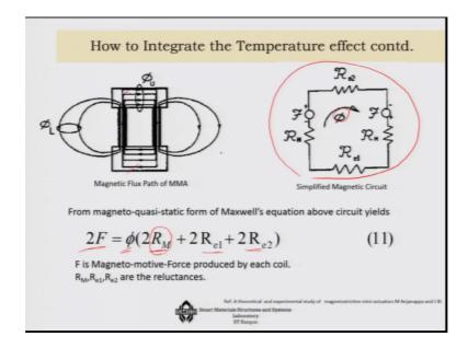
the only now is that you earlier remember the expression of blocking force now the magnetic point of view the from the Maxwell's equation the magnetomotive force can be written in terms of magnetic flux and in terms of the reluctances of the system ok.
