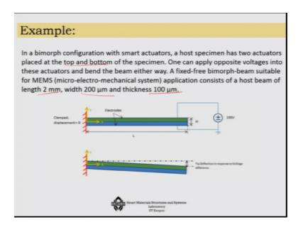
So, let us try to discuss this whole concept with the help of an example. The example that we have chosen is that of a bimorph ok. So, you can see a bimorph here and in this by bimorph, what you have is a you know piezoelectric material 2 piezoelectric layers which are joined together. 2 actuators placed at the top and bottom of the specimen and we can apply opposite voltage to each one of them.
