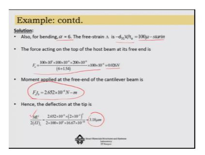
Now, for bending we know that alpha is equals to 6 and free strain lambda is also known to us. We can find it out because the voltage is known to us which will give us lambda to be 100-micron strength. So, you can use this data and we can find out what is the force that is acting on the top of the host beam which will come out to be 0.026 Newton exactly an opposite force is there in the bottom. So, this actually comes up in the form of a couple.
