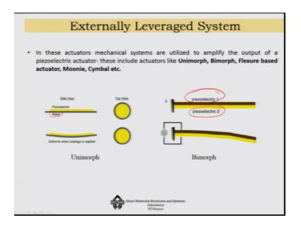
The other way is to go for externally leverage system ok. So, say for example, the simple you know Unimorph systems or in which one part is piezoelectric another part is metal that is uniform or both are Piezoelectric. And you apply opposite voltage that is the Bimorph system or you can have this kind of system which is flexure based ok.
