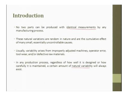
So, now let us get into the topic of discussion for limits fits and tolerance. So, introduction no, two parts can produce with identical measurements by any manufacturing process, any process or any event to happen follow the binomial distribution right. So, if that is the case then any two parts produced if you want to make it as accurate as possible they it is next to impossible. So, there is no manufacturing process in this world, which can make two products very identical.
