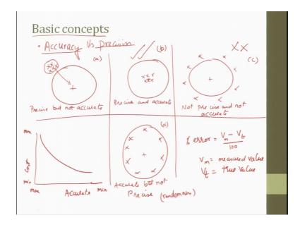
Ok based on some of the queries which are raised by the students I would like to explain first a basic concept called accuracy and precision though I gave you only the definition now I will give it with respect to a figure, so that you can appreciate it.
