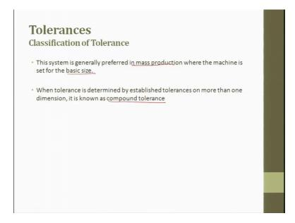
So, this system is generally preferred in mass production where the machine is set to the basic size. The tolerance is determined by establishing tolerance on more than one dimension it is known as compound tolerance. So, we will continue it in the next lecture what is compound tolerance and continue.
