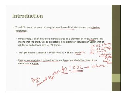
The difference between upper and lower limit is termed as permissible tolerance so I tolerate I tolerate, so that is why it is called as tolerance. I tolerate the variations that is why it is called as tolerance. For example, a shaft has to be manufactured to the diameter of 40 plus or minus 0.02 millimeter, this means that the shaft will be accepted if the diameter between the upper limit of 40.02 and lower limit of 39.98.
