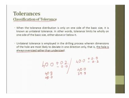
Next is let us start looking into classification of tolerance, when the tolerance distribution is only on one side of the basic size it is known as unilateral tolerance, in the other words the tolerance limit lies wholly on one side of the basic side either above or below, unilateral tolerance is employed in drilling process wherein with. So, what is that let us see so, it is 40.0 I say plus that is all or I can say plus minus 0.0.
