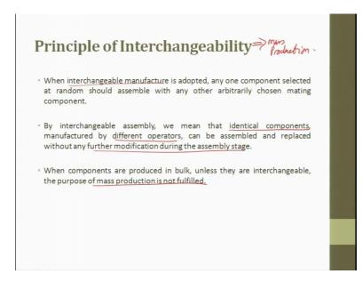
This gave a big revolution, when interchangeability of manufacturing is adopted, any one component selected at random should assemble with another with any other arbitrary chosen mating component. So, I have a nut a box of nut is there I pick one nut I take a box a counter say for example, M 6 nut I take and I have a big box of 1000s bolt I pick
