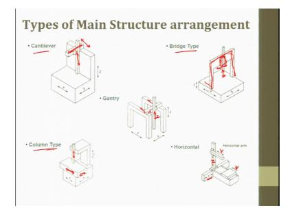
Types of main structure arrangements in the CMM machine or cantilever you know this is a cantilever beam the cantilever beam is moving in X direction, cantilever beam can move in X direction and on this cantilever beam we have this arm that can move in Z direction. So, second one is column type, in column type we have the table that can move here this table can move in X and Y direction in Z direction this arm can move ok.
