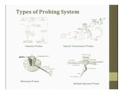
So, different types of probing systems are there we have inductive probing system like we have inductive probing system we have machining center arrangement. So, inductive or inductive transmission is the principle in using this probe, then optical transmission probe there when optical transmission is a principal. Similarly, we have motorized probes motorized probes in which just we have the motors and motors can just rotate the probe or move the probe.
