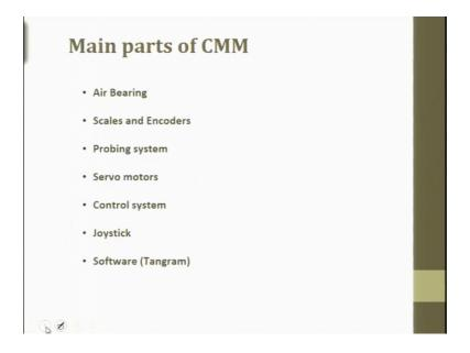
So, main parts of CMM are air bearing I will show this parts do there. So, we have pneumatic bearings here so, then scales and encoders, probing system servo motors which are just making the past to move. So, control system is here, joystick is here, software is here, software that we use here Tangram software ok.
