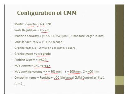
So, the single machine that we have here, I will the configuration of that is it is spectra 5 6 4. What is 5 6 4? 5 is 500 and 600 and 400 is the work area or the workspace that is available in the 3 axes, 500 mm, 600 mm 400 mm ok.
