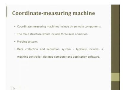
So, coordinate measuring machine include 3 major components, number 1 is the main structure with include 3 axes of motion X, Y and Z axis number 2 is the probing system as I said we have a mechanical probing system here. Number 3 is the data collection and reduction system, data collection data reduction means we clean the data, data cleaning ok. So, this typically includes a machine controller machine controller is your UCC, desktop computer and application software.
