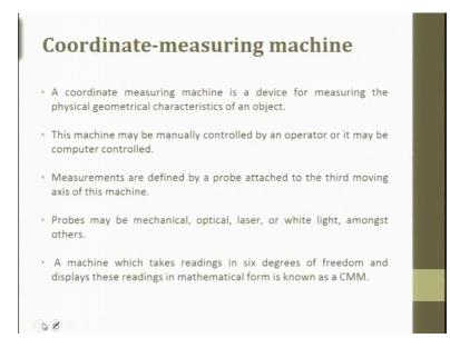
Now, I like to move to a coordinate measuring machine a coordinate measuring machine is a device for measuring the physical geometrical characteristics of an object this I have just explained. To this machine may be manually controlled by an operator or it may be computer control so, will show you the both operations, the manual control using a joystick and CNC mode as well. CNC mode is computer numerical control. We just give the initial point of it this is the starting point.
